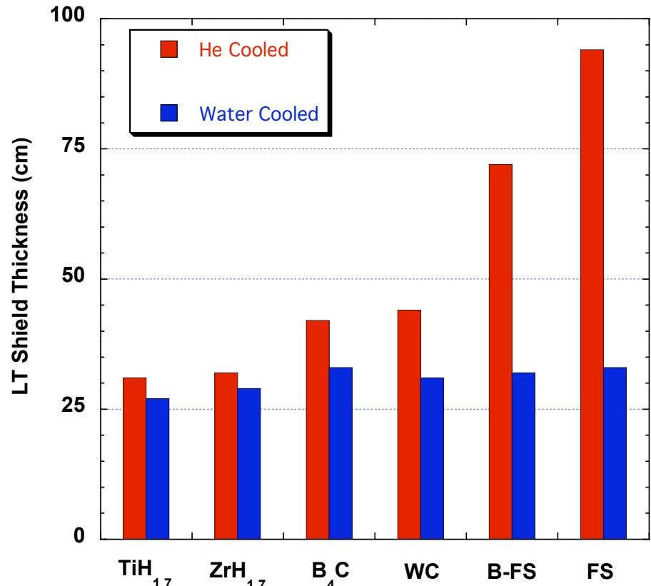
For non-hydride fillers, water reduces LT shield size significantly
