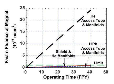
High n fluence behind He access tubes degrades  $J_c$  of superconductor
