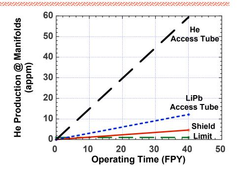
He production at manifolds is excessive
