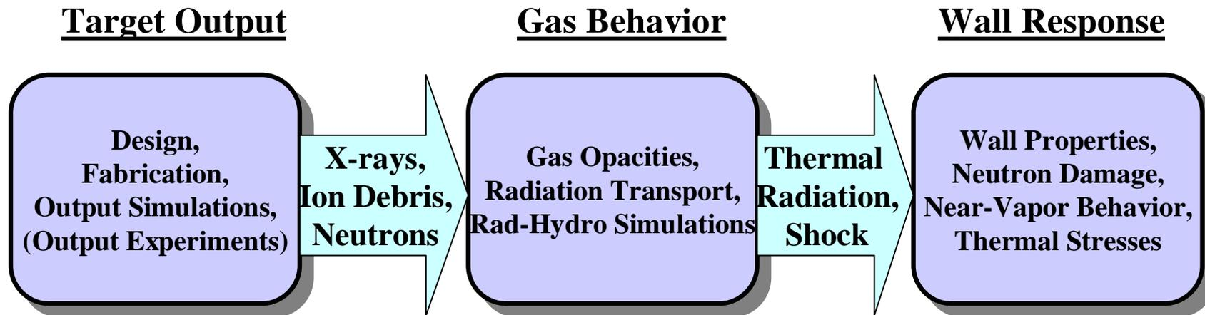
UW uses the **BUCKY** 1-D Radiation-Hydrodynamics Code to Simulate Target, Gas Behavior and Wall Response.
