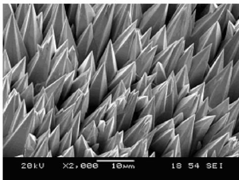
Re dendritic coating on W substrate
