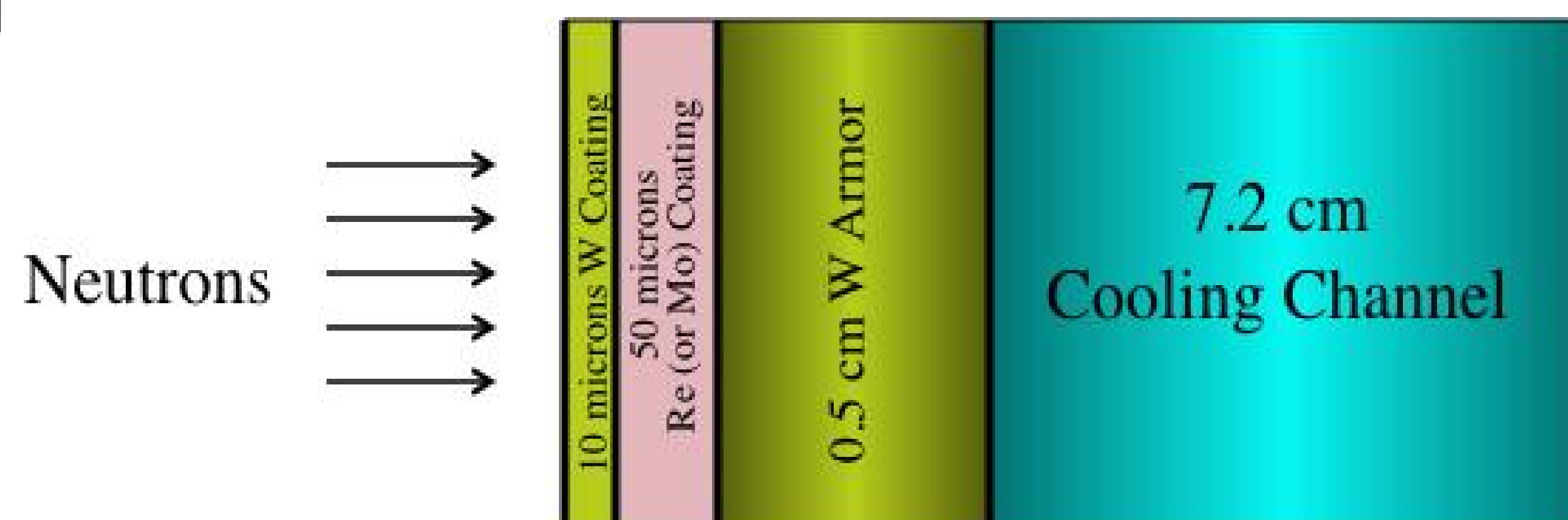
Radial build of divertor model for WDR calculations given Re and Mo coatings of thicknesses varying from one to 50 microns.
