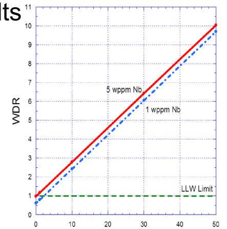
WDR as function of thickness for Mo coating given tungsten Nb impurity content of 1 and 5 wppm.
