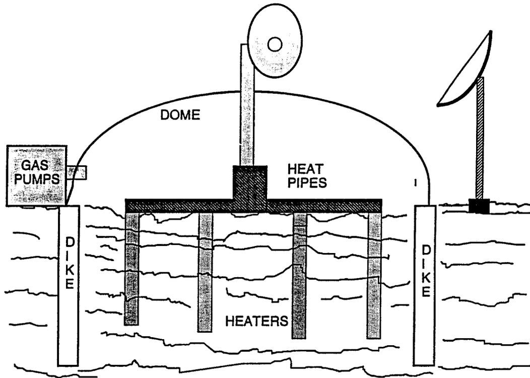
Figure 2. Conceptual design of an in-situ technique to evolve volatiles from the lunar regolith. Pneumatic structures are used to contain the gases and an artificial  $H_2$  atmosphere. Small heaters, utilizing solar energy, are placed vertically in the soil.
