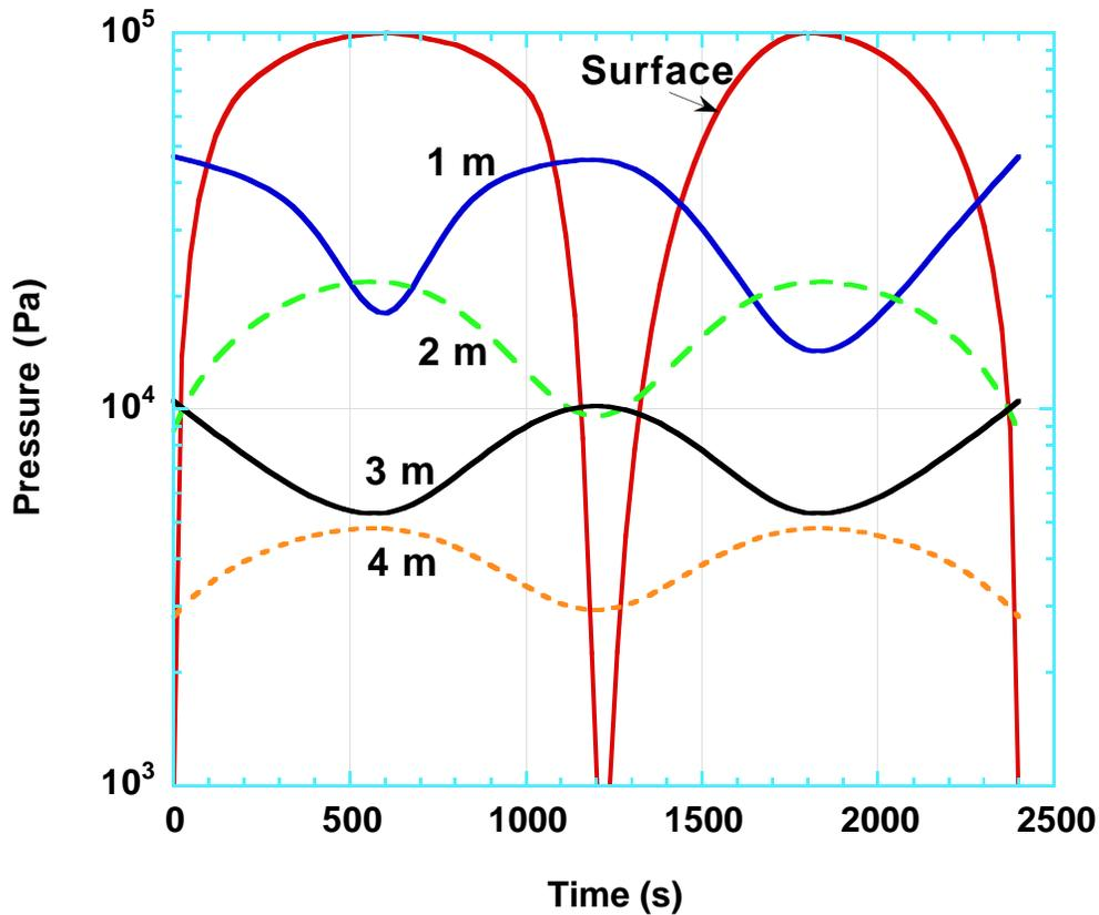
Figure 3. Periodic hydrogen pressure at several depths in the regolith as a function of time.
