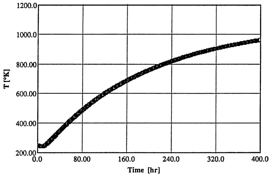
Figure 1. Temperature increase of the soil as a function of time at the boundary between two cylindrical soil configurations of 0.5 m radius with the axis of each cylinder maintained at 1073°K.
