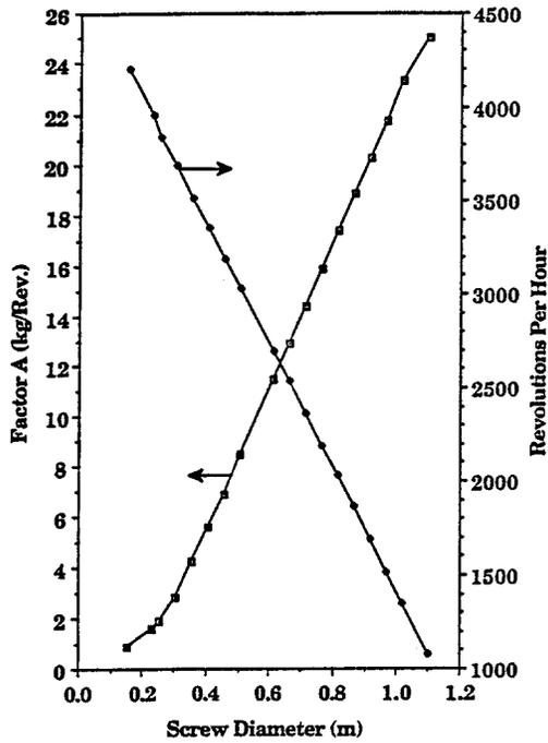
Figure 4. Factor A and allowable RPH as a function of screw diameter.
