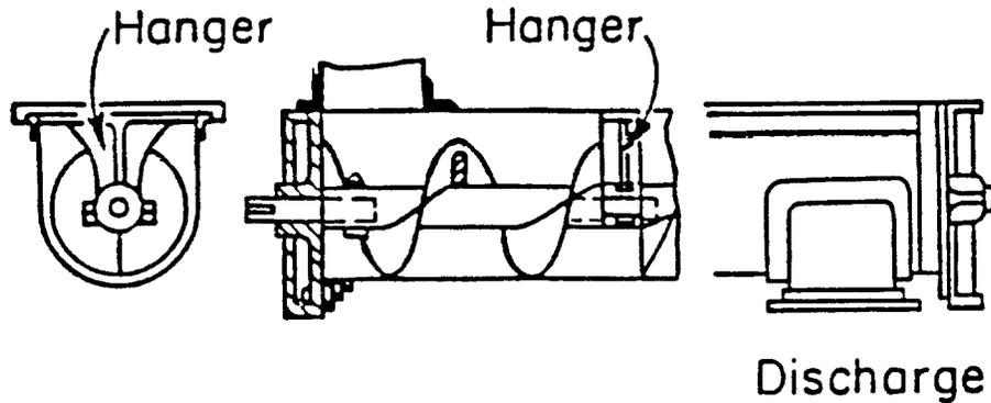
Figure 3. A typical power screw conveyer system.
