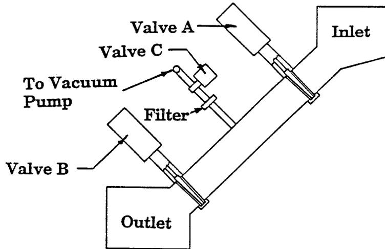
Figure 2. A system for a batch process conveyer.
