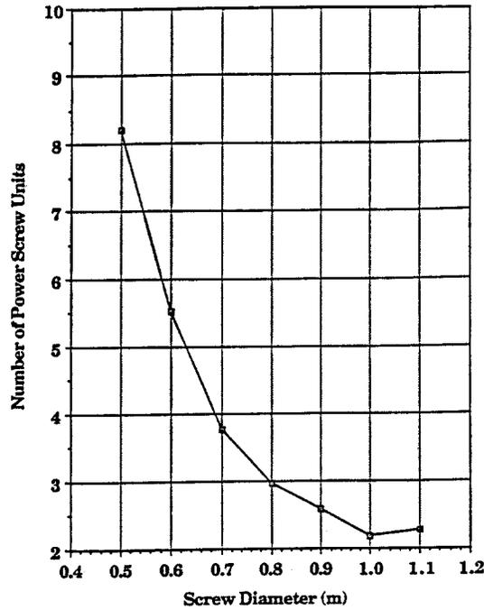
Figure 5. Number of power screws needed to convey 310 m<sup>3</sup>/h of lunar fines as a function of screw diameter.
