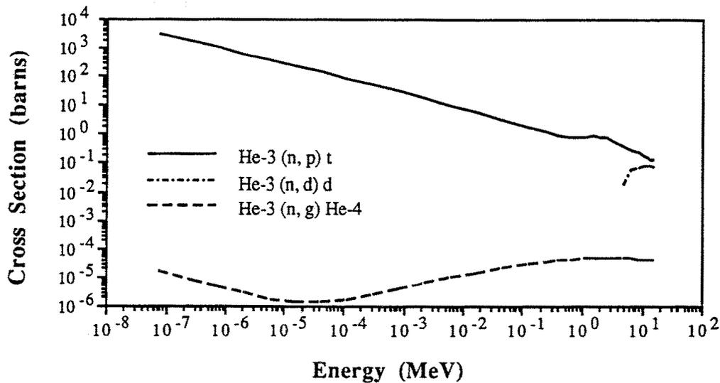
Figure 1. Possible  $^3\text{He}$  - neutron interaction cross sections (National Nuclear Data Center, BROND-2 data base).
