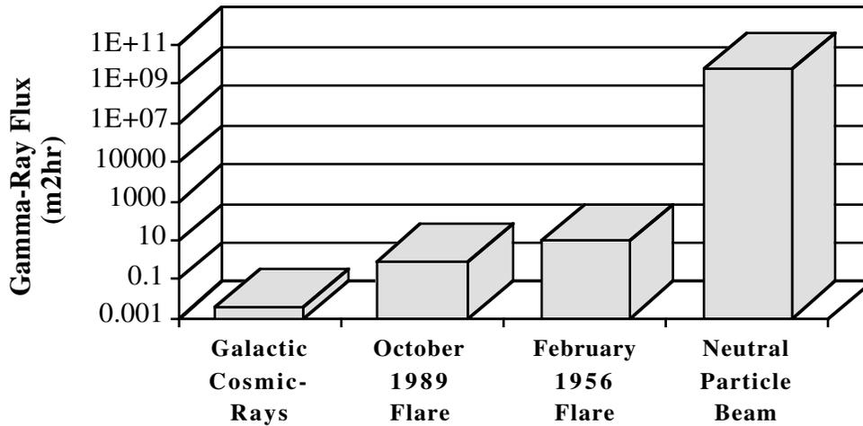
Figure 6. The 20.6 MeV gamma-ray flux from lunar <sup>3</sup>He calculated from various neutron sources. Note that the gamma-ray source from the NPB is a point source at the lunar surface.
