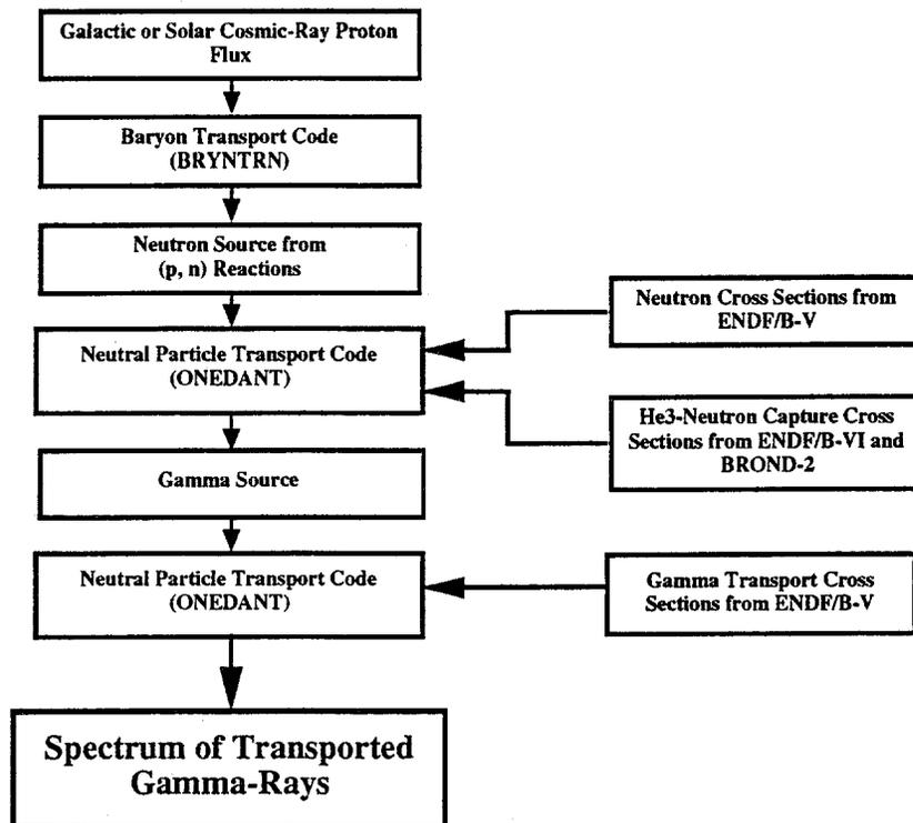
Figure 4. Flow chart of the computational method used in calculating the gamma-ray flux from  $^3\text{He}$  due to an incident proton flux.
