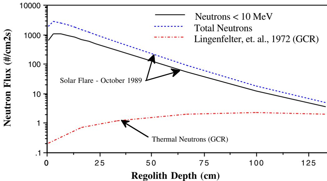
Figure 5. Neutron flux as a function of depth for the October 1989 VLSPF as calculated using BRYNTRN. The thermal neutron flux is that calculated by Lingenfelter et al. (1972) [7].
