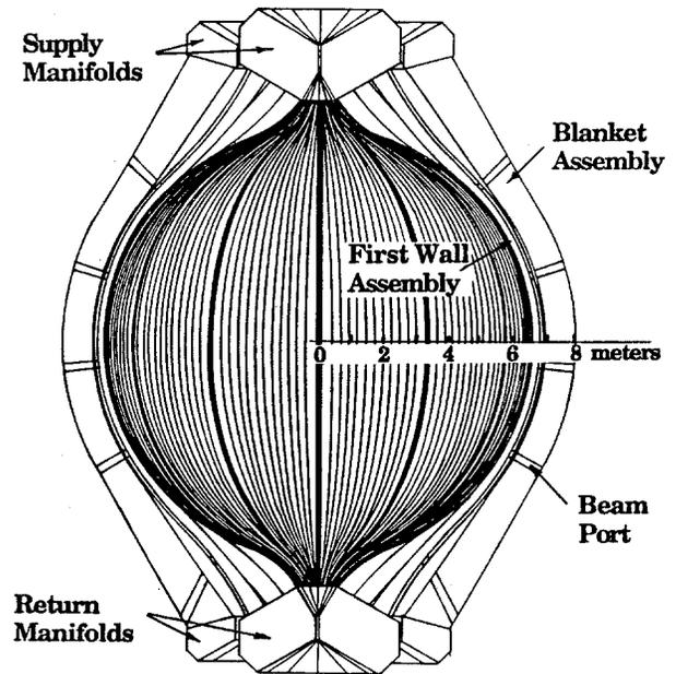
Fig. 2. Cross section of SIRIUS-P reactor.
