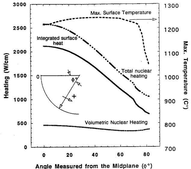
Fig. 3. Maximum FW surface temperature and nuclear heating in lower half of SIRIUS-PR chamber.
