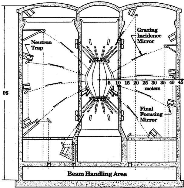
Fig. 1. Side view of containment building.
