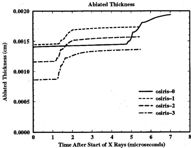
Fig. 1. Ablated thickness in OSIRIS type chambers.
