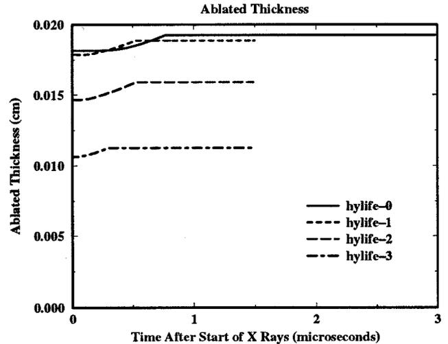
Fig. 2. Ablated thickness in HYLIFE-II type chambers.
