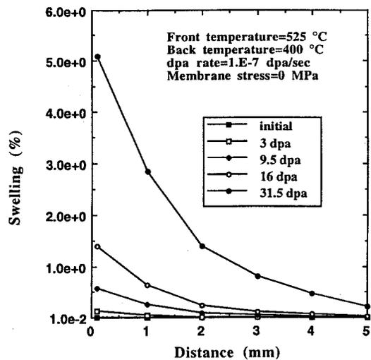
Fig. 9. Evolution of the stress-enhanced swelling distribution as a function of dpa for a 5 mm 316 SS plate.
