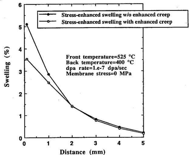
Fig. 10. Effect of (stress-enhanced swelling)-enhanced creep on the swelling of a 5 mm 316 SS plate after 31.5 dpa.
