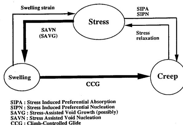
Fig. 1. Relationship between Swelling-Creep-Stress in a radiation environment.
