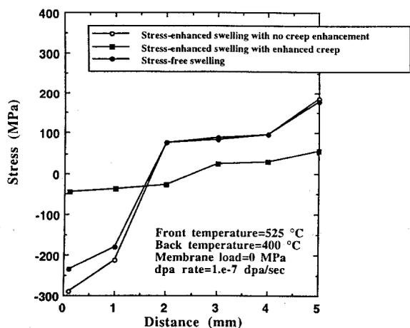
Fig. 11. Effect of stress-enhanced swelling with enhanced creep on the stress distribution in a 5 mm 316 SS plate after 31.5 dpa.
