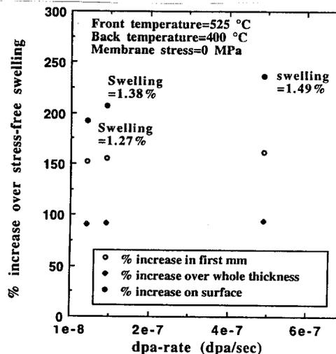
Fig. 3. Effect of dpa rate on the stress-enhanced swelling behavior of 5 mm 316 SS plate after 15.75 dpa.
