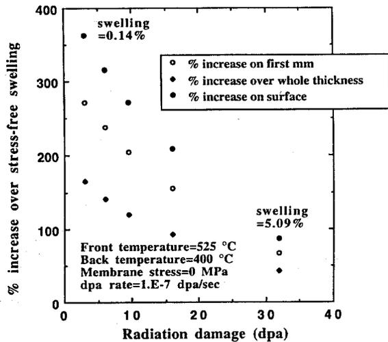
Fig. 7. Effect of stress on swelling behavior of a 5 mm SS plate as a function of radiation dose.
