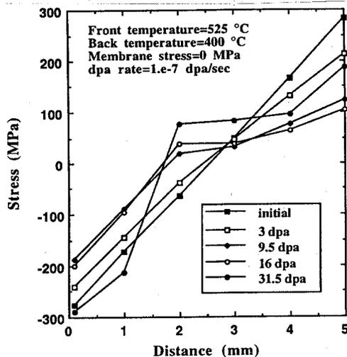
Fig. 8. Evolution of stress as a function of dpa for a 5 mm 316 SS plate.
