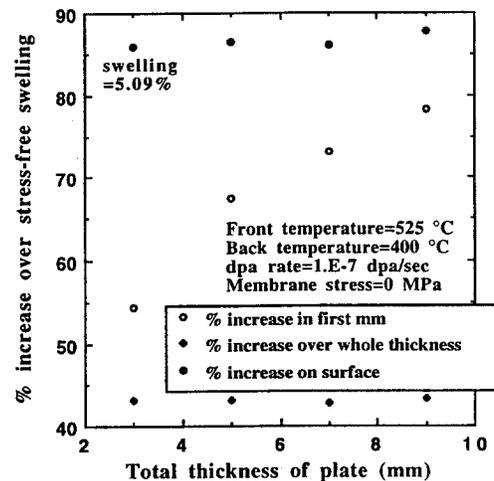
Fig. 2. Effect of plate thickness on the stress-enhanced swelling of 316 SS plate after 31.5 dpa.
