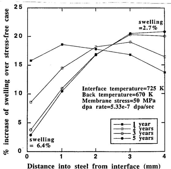
Fig. 12. Percentage increase in stress enhanced swelling over the stress free case for a 20% cw 316 SS substrate coated with 2 mm of Be.
