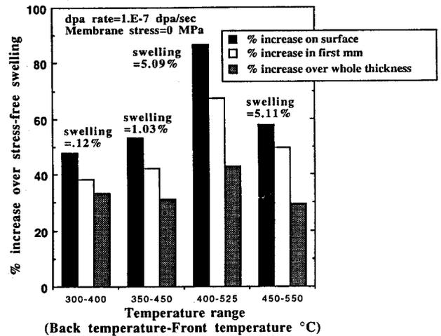
Fig. 6. Effect of temperature range on the stress-enhanced swelling behavior of a 5 mm 316 SS after 31.5 dpa.
