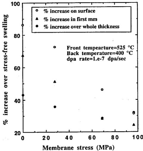
Fig. 4. Effect of membrane stress on the stress-enhanced swelling of a 5 mm 316 SS plate after 31.5 dpa.
