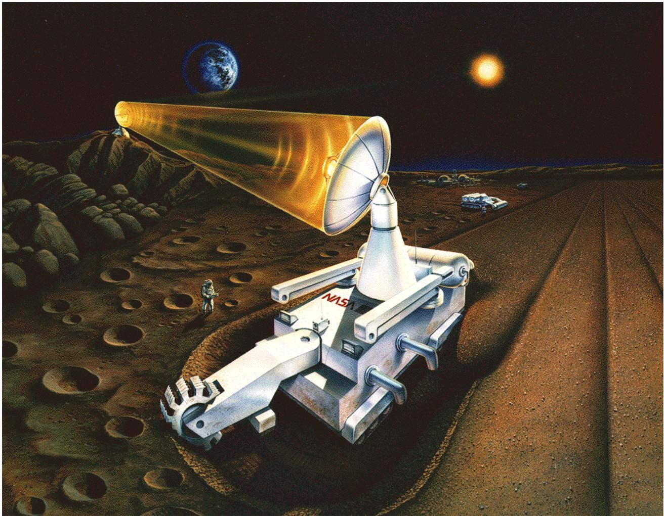
Fig. 6. An artist's conception of a lunar miner at work on the Sea of Tranquillity. Note the solar relay mirror which beam energy to the slowly moving miner for heating the regolith. This unit could supply the  $^3\text{He}$  fuel for a city of 500,000 people in the U.S.
