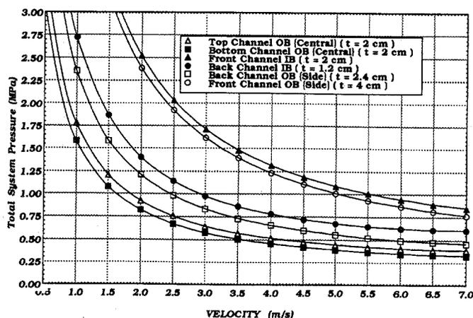
Fig. 2. Effect of velocity on pressure.
