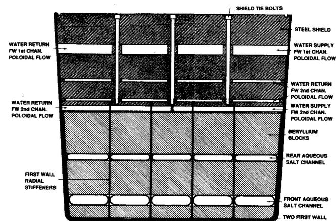
Fig. 1 Outboard side module midplane cross section.
