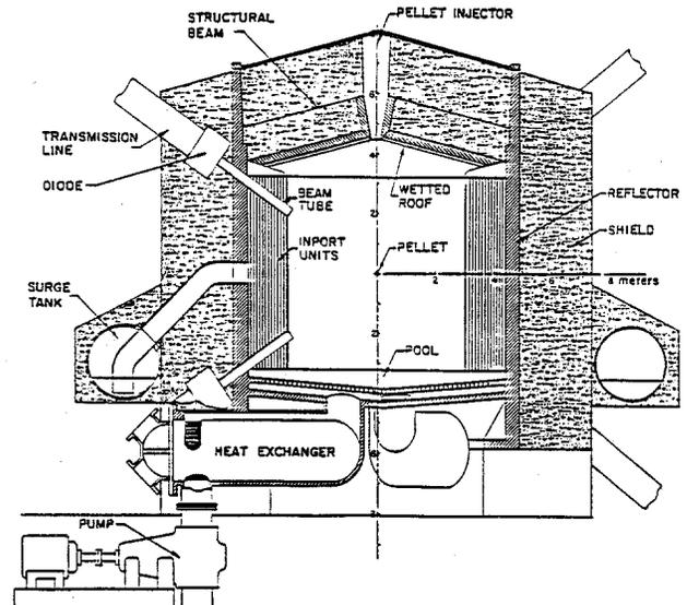
Fig. 1. Cross Section of Target Chamber.
