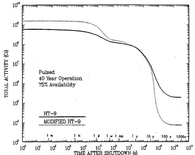
Fig. 4. Effect of Low Activation Structure on Total Activity in LIBRA Chamber.
