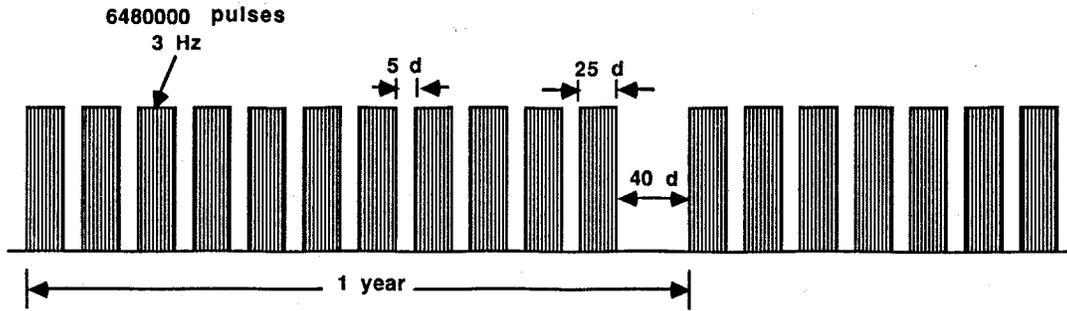
Fig. 2. Pulse Sequence Used in the LIBRA Activation Calculations.
