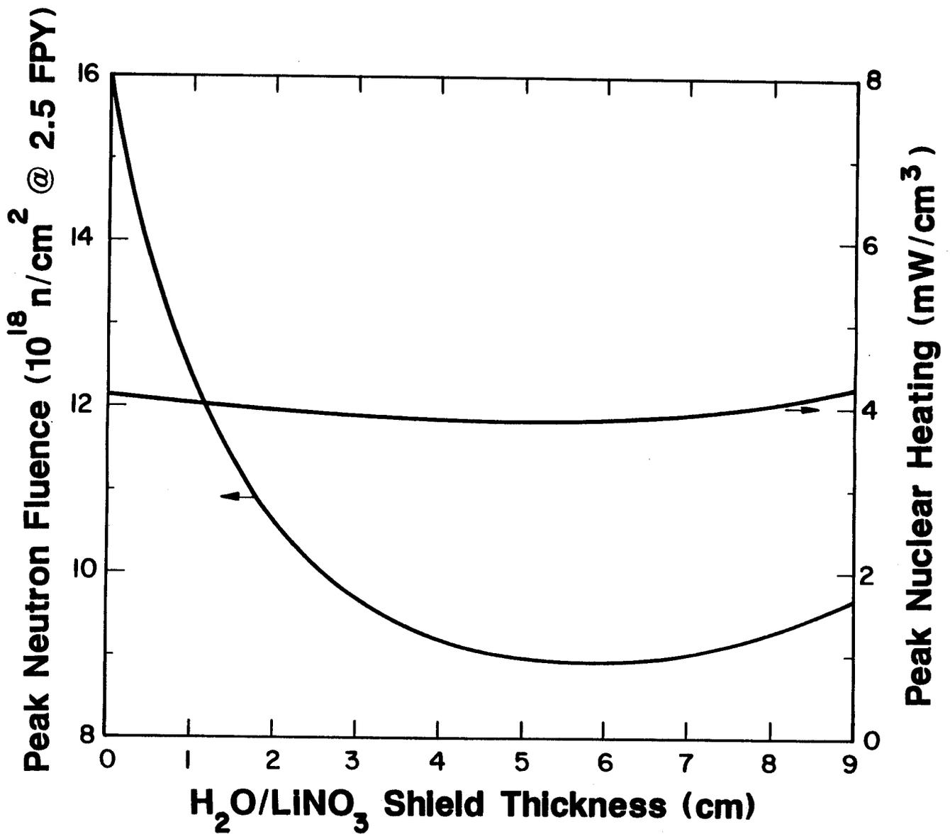
Fig. 4. Variation of the radiation effect in the coil with the H<sub>2</sub>O/LiNO<sub>3</sub>-shield thickness.
