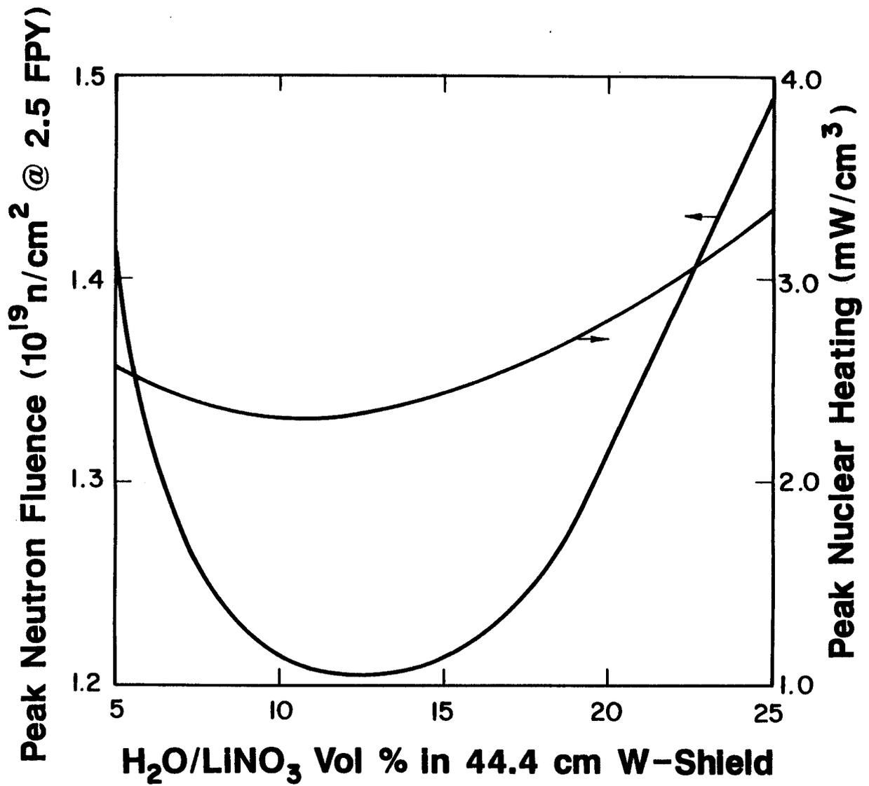
Fig. 2. Effect of trading H<sub>2</sub>O/LiNO<sub>3</sub> for W on damage in magnet.
