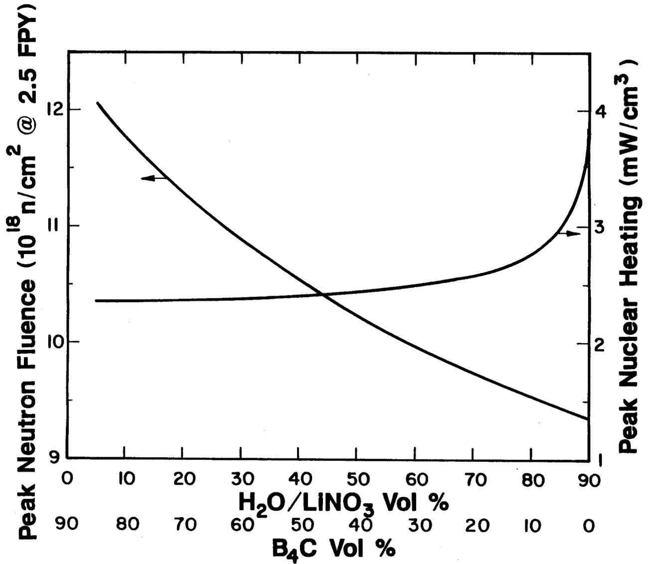
Fig. 3. Effect of trading B<sub>4</sub>C for H<sub>2</sub>O/LiNO<sub>3</sub> in 3.6 cm thick back layer of B<sub>4</sub>C-shield.
