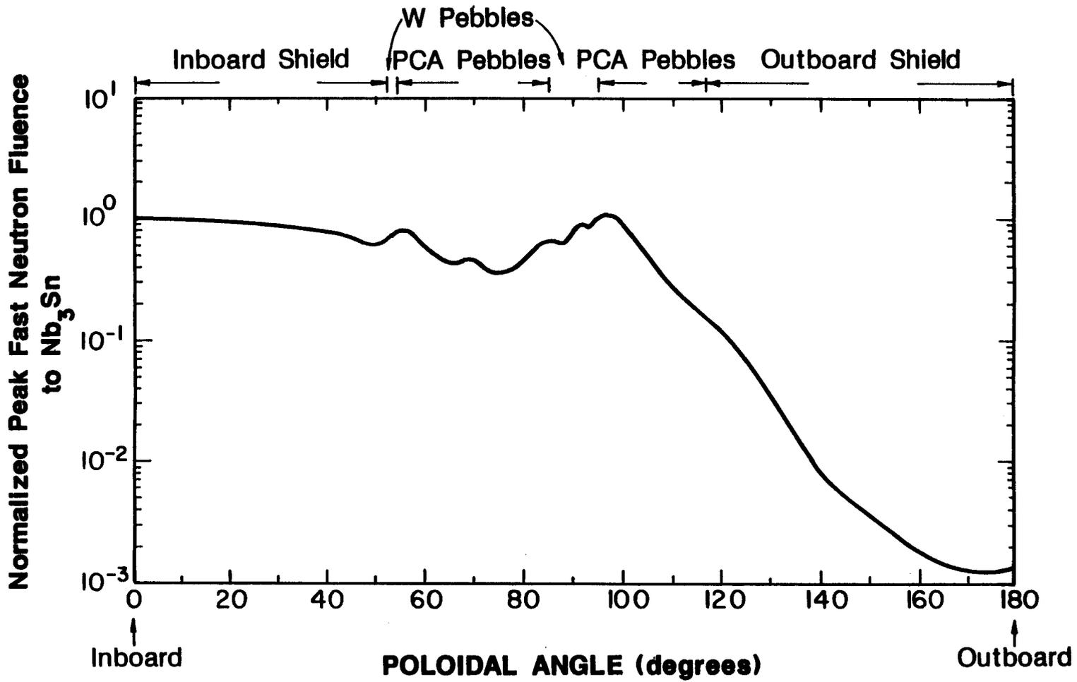
Fig. 7. Poloidal variation of the fluence in the TF coils.
