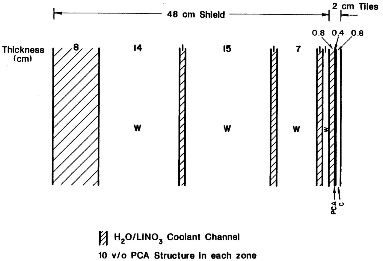
Fig. 6. Layered i/b shield configuration.
