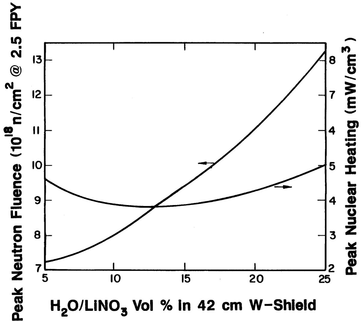
Fig. 5. Effect of trading H<sub>2</sub>O/LiNO<sub>3</sub> for W on damage in magnet.
