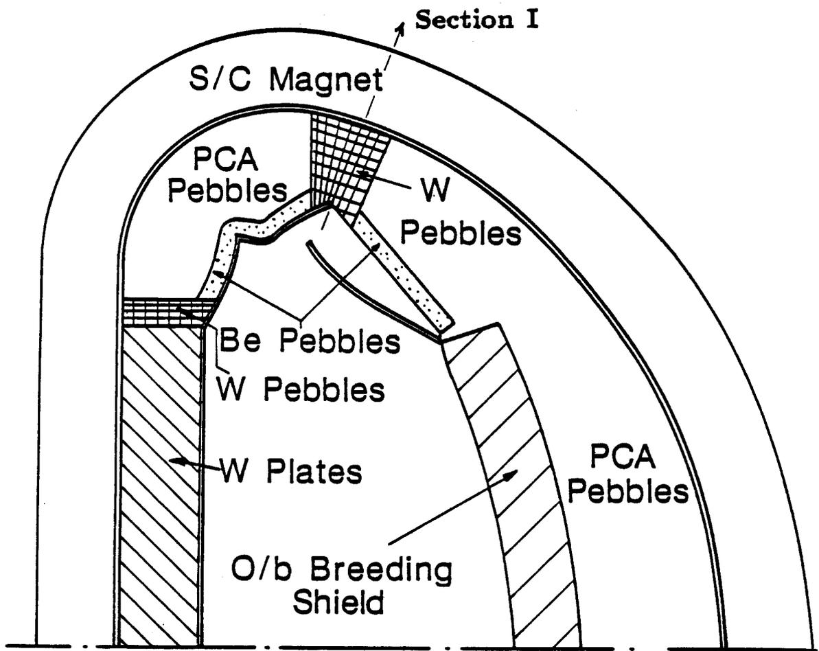
Fig. 1. A cross section through the TF coil of TIBER-II showing the different zones of the shield.
