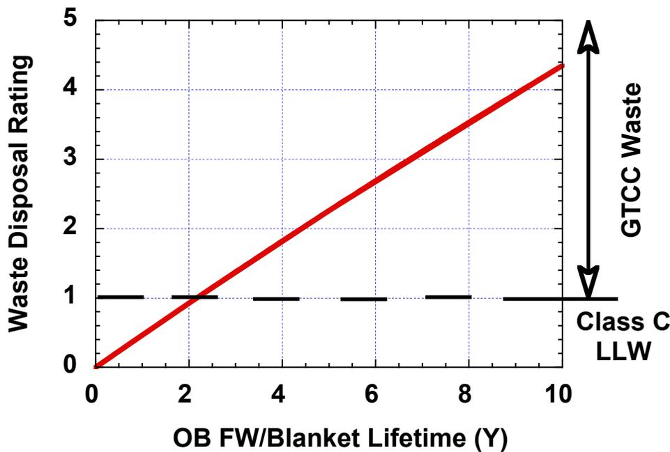
Figure 5. Reduction of WDR with OB FW/blanket service lifetime for ODS 125Y structure.
