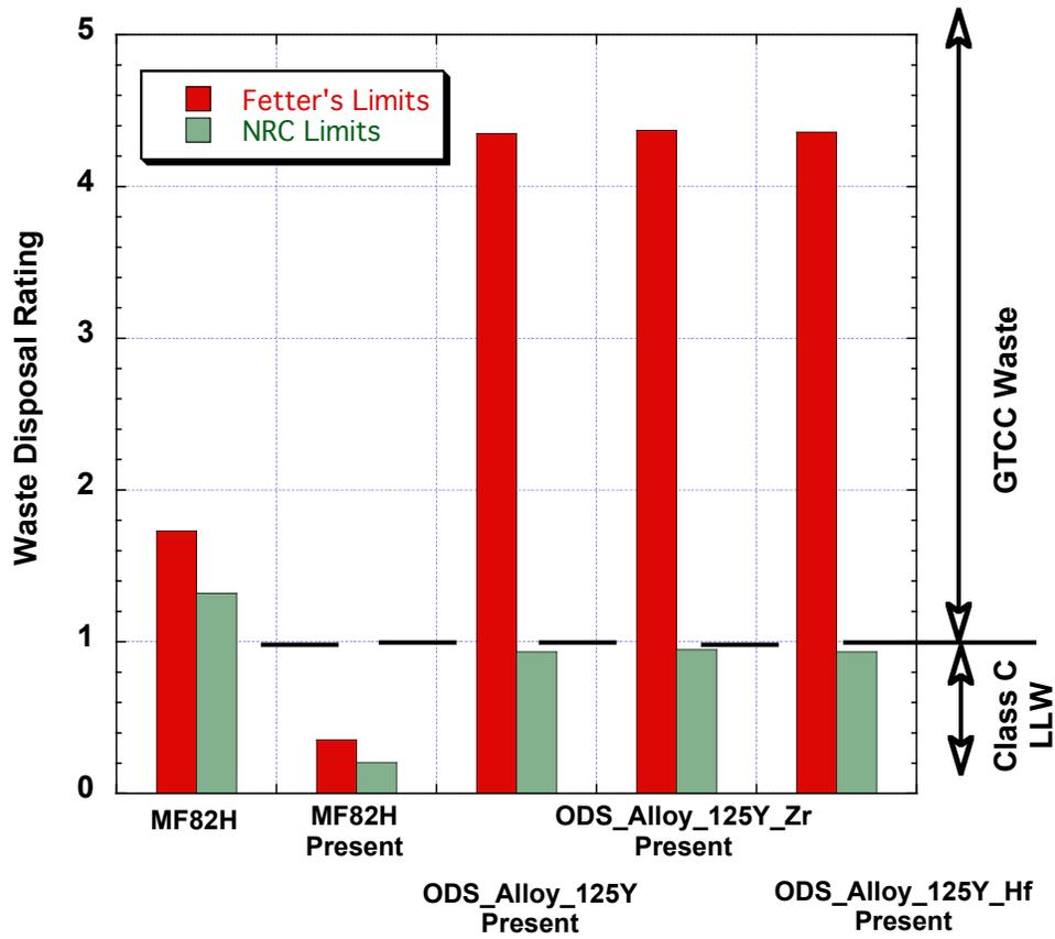
Figure 4. Waste disposal rating of fully compacted FW/blanket after  $\sim 13 \text{ MWy/m}^2$  of irradiation. Red bars for WDR using Fetter's limits. Green bars for WDR using NRC limits.
