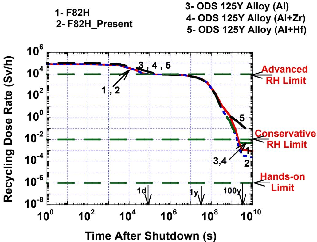
Figure 2. Time variation of recycling dose rate to the RH equipment for the OB FW of ARIES-ACT-2 design using corrosion-resistant ODS alloys. The F82H alloy is included for comparison.
