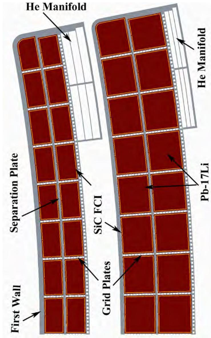
Fig. 1. Midplane cross section of outboard DCLL blanket of ARIES-ACT-2 showing the 40 cm thick inner blanket segment (that includes the 3.8 cm thick FW), 60 cm thick outer blanket segment, PbLi flow channels (in brown), cooling channels (in grey), and SiC FCI (in orange).
