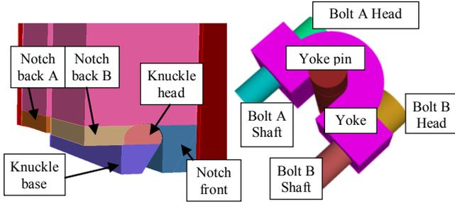
Figure 3. Detailed view of regions of interest for nuclear heating analysis.
