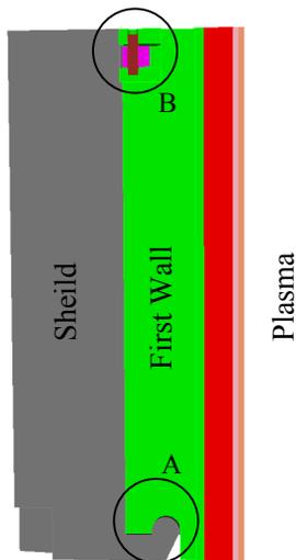
Figure 1. Cross-section through middle of Module 4 prototype showing (A) hinge and (B) yoke/pin attachment.
