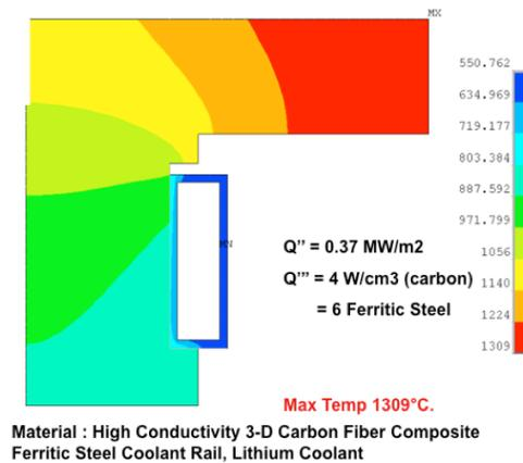
Figure 7. Temperature distribution in FW tile at mid-plane.
