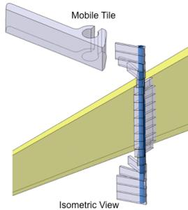
Figure 3. Tile configuration at laser beam ports.
