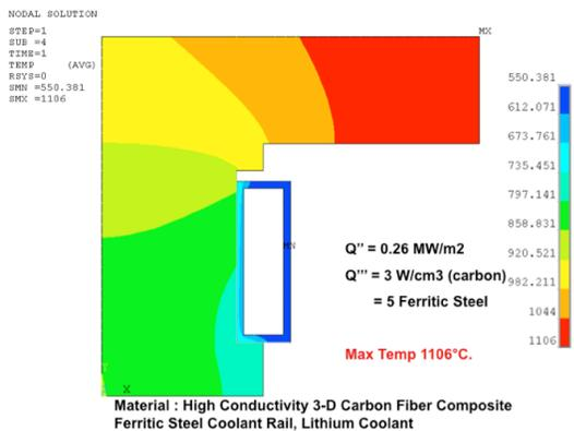
Figure 8. Temperature distribution at average FW tile conditions.
