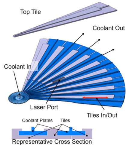
Figure 5. Configuration of top tiles.
