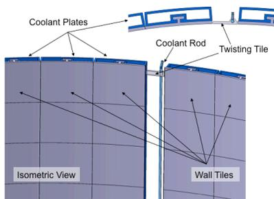
Figure 4. Overall configuration of tiles on chamber side wall.
