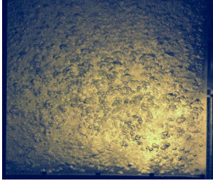
Fig. 3. Water with 15% void fraction of argon in a mock-up of the shock tube test section with transparent walls—the width of the test section is 25.4 cm.
