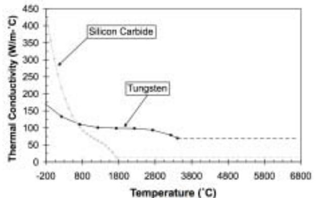
Fig. 1. Thermal conductivity of tungsten and silicon carbide.
