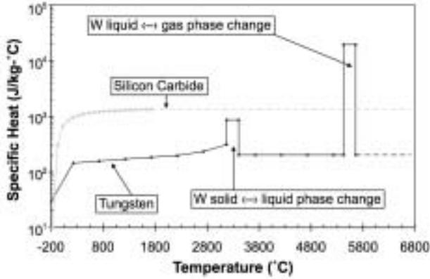
Fig. 2. Specific heat of tungsten and silicon carbide.
