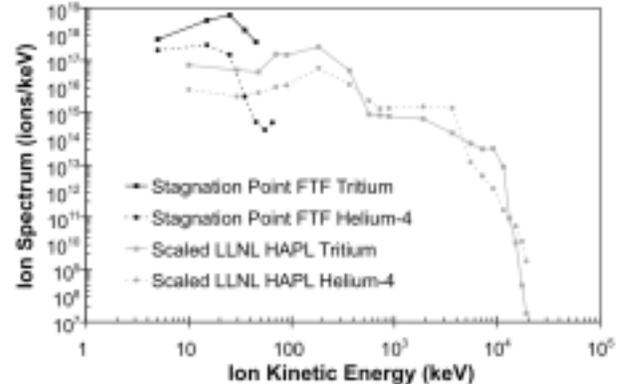
Fig. 9. Tritium and Helium spectra from the scaled HAPL and compressed FTF targets.
