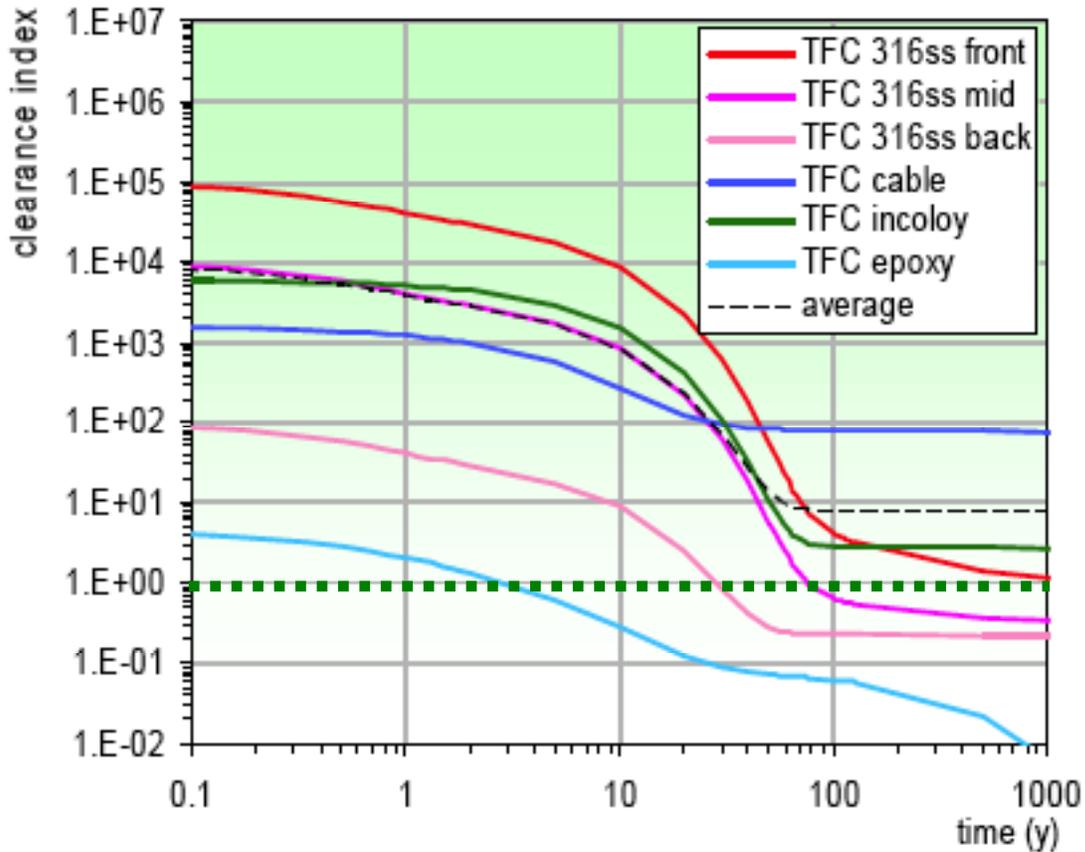
Fig. 3. CI time histories of the different TFC materials at the inboard midplane of PPCS-AB.
