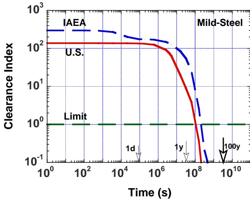
Fig. 6. Comparison of U.S. and IAEA clearance indices for steel of innermost segment of bioshield.
