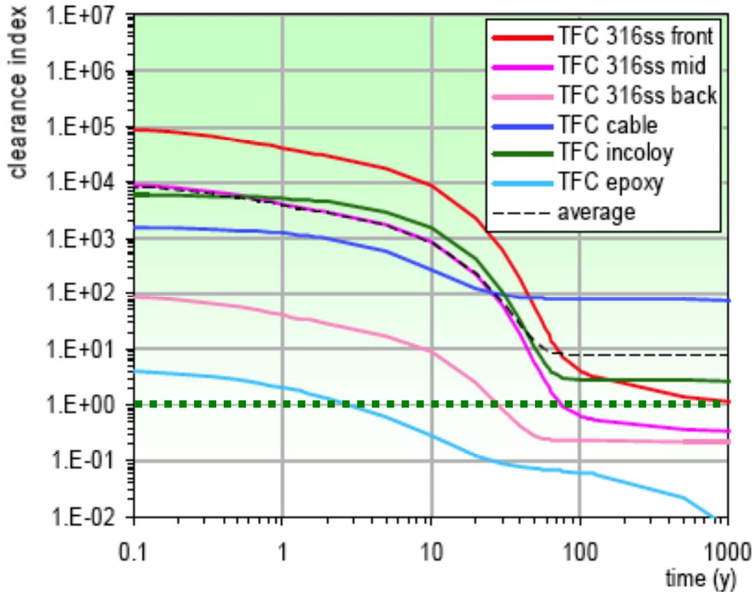
Fig. 10. CI time histories of the different TFC materials at the inboard midplane of PPCS-AB.
