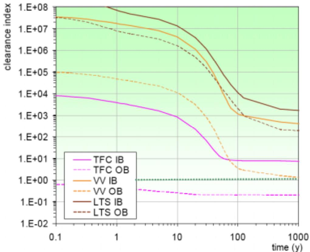
Fig. 8. CI time histories of lifetime components in PPCS-AB, at inboard and outboard midplane.
