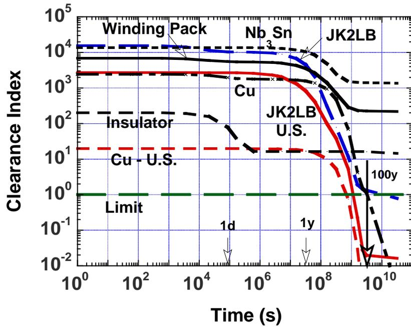
Fig. 5. Variation of IAEA CI of winding pack constituents with time after decommissioning. The U.S. CI for JK2LB steel and Cu stabilizer are included for comparison.
