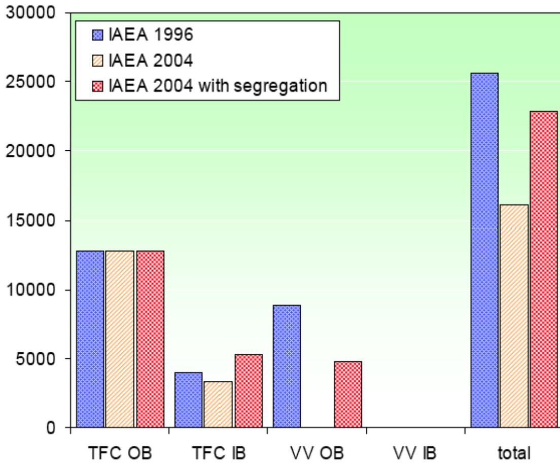
Fig. 11. Amounts of clearable material in PPCS-AB under (a) IAEA 1996 levels, (b) IAEA 2004 levels, and (c) IAEA 2004 levels applying segregation of materials.
