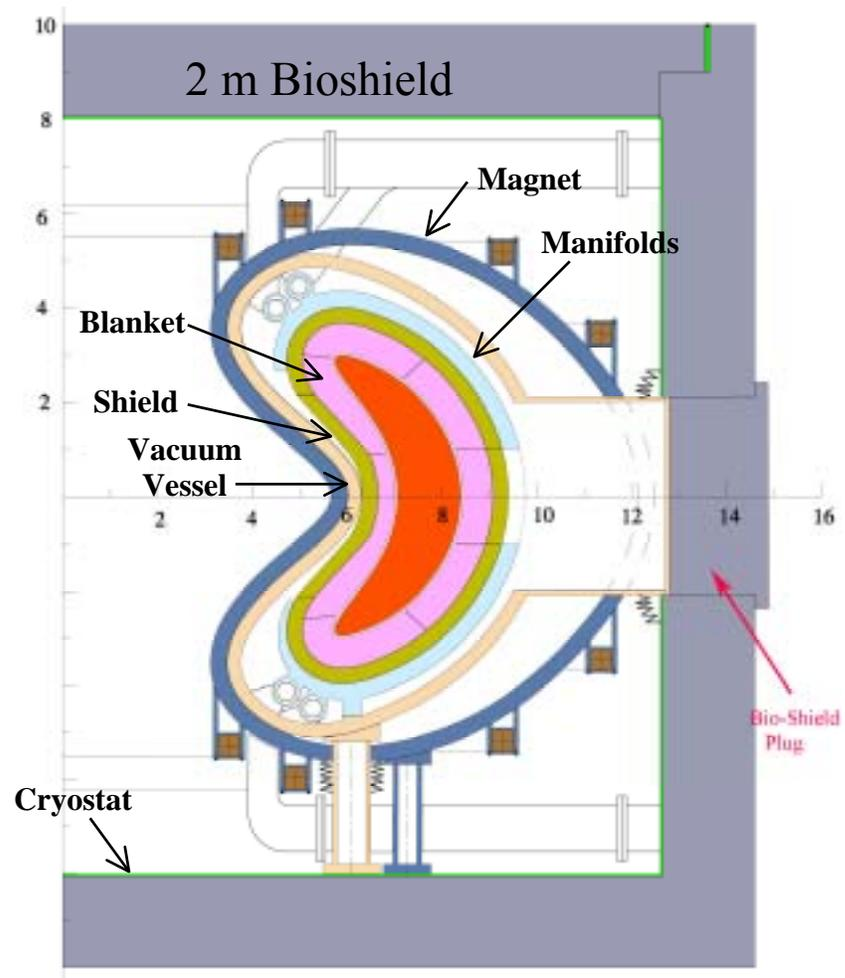
*Fig. 3. Vertical cross section of ARIES-CS showing the main core components and the surrounding cryostat and bioshield.*
