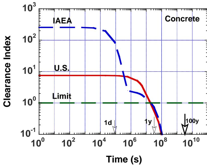
Fig. 7. Comparison of U.S. and IAEA clearance indices for concrete of innermost segment of bioshield.
