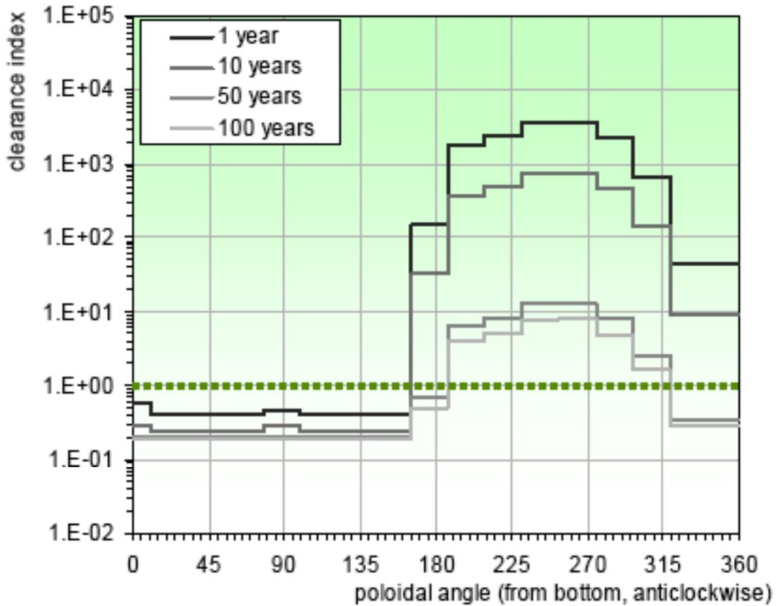
Fig. 9. Poloidal variation of the TFC CI in PPCS-AB at different times after shutdown.
