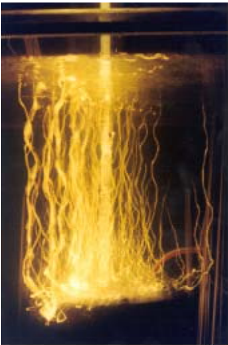
Figure 5. Time-exposed photograph of the coarse fragmentation of a 9 mm-diameter drop of molten ferrosilicon alloy in water at 83 °C. (C-203-1-6)
