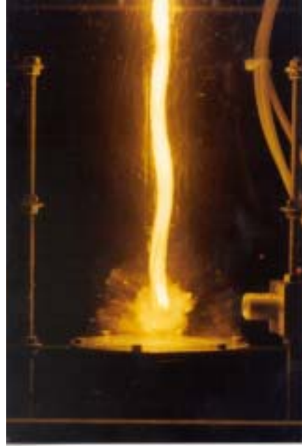
Figure 4b. Time-exposed photograph of the steam explosion of a 9 mm-diameter drop of molten silicon. (D-59-1-2)
