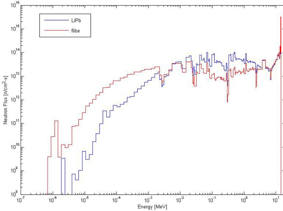
Fig. 1. MCNP calculated neutron flux at RTL for Flibe and LiPb breeder options.
