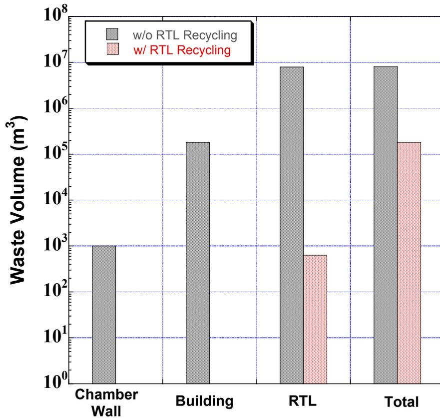
Fig. 2. RTL inventory and waste comparison.
