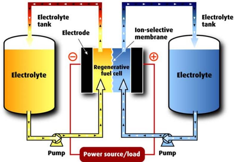
**Figure 9: Flow Battery**
