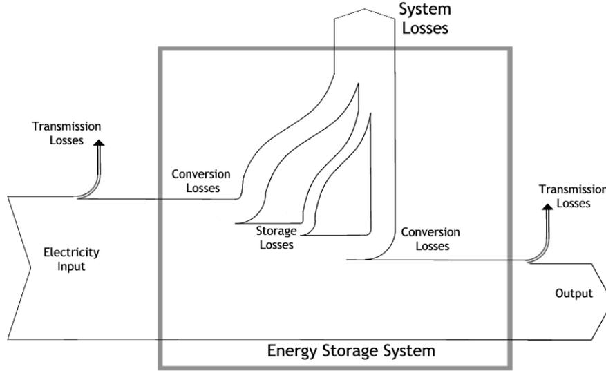
**Figure 4: Energy Flow in an Energy Storage System**
