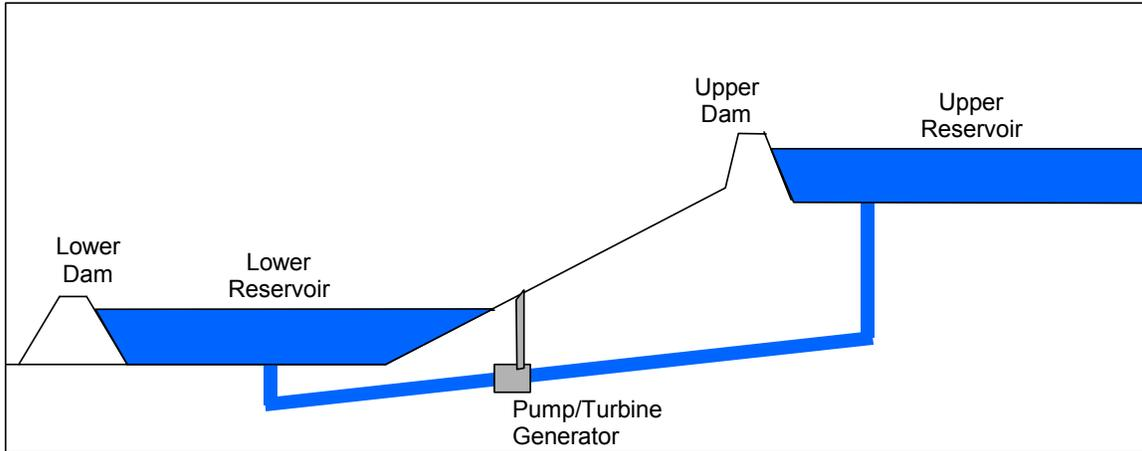
**Figure 5. Pumped Hydro Storage**
