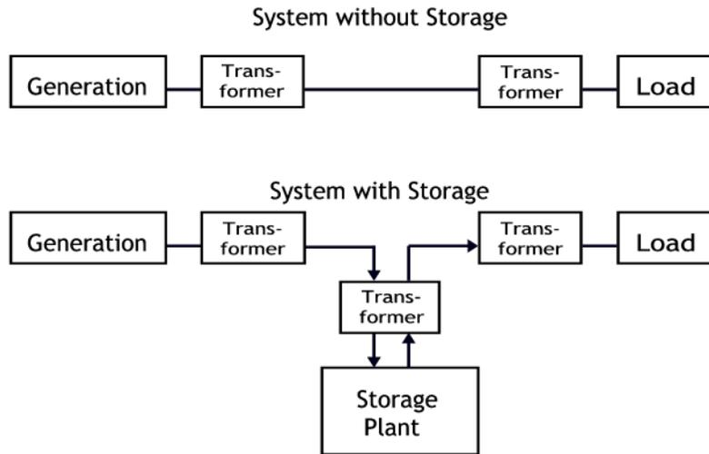
**Figure 3: Additional Transmission Components Required by Energy Storage**
