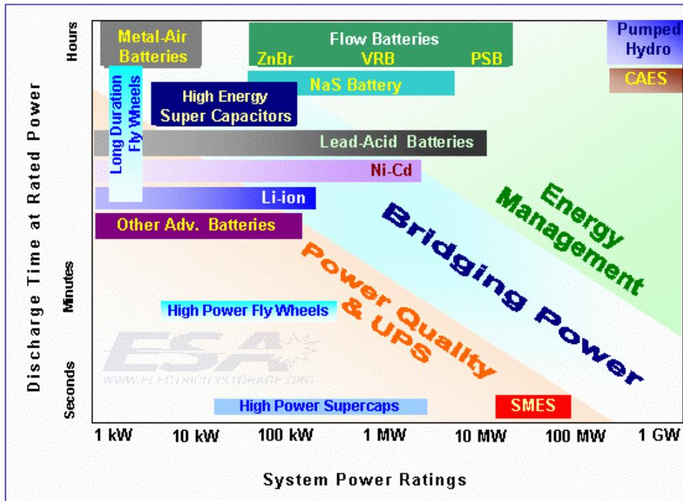
**Figure 1: Power and Energy Ratings for Currently Available Energy Storage Technologies**
