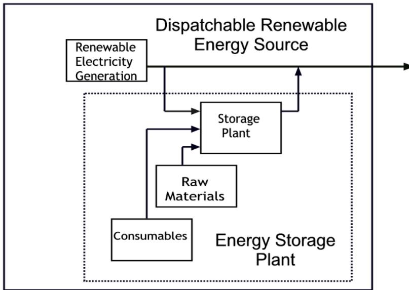
**Figure 2: System Boundaries for an Energy Storage System and a Dispatchable Renewable Energy Source**
