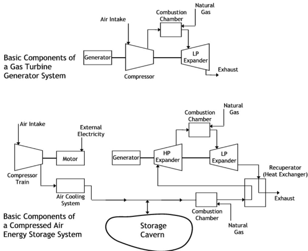
**Figure 6: Schematic Diagrams of Gas Turbine Generation and Compressed Air Energy Storage**
