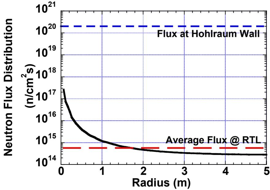
Figure 7. Radial distribution of the neutron flux in the 5 m Z-pinch chamber. The flux at the HI hohlraum wall is shown for comparison.
