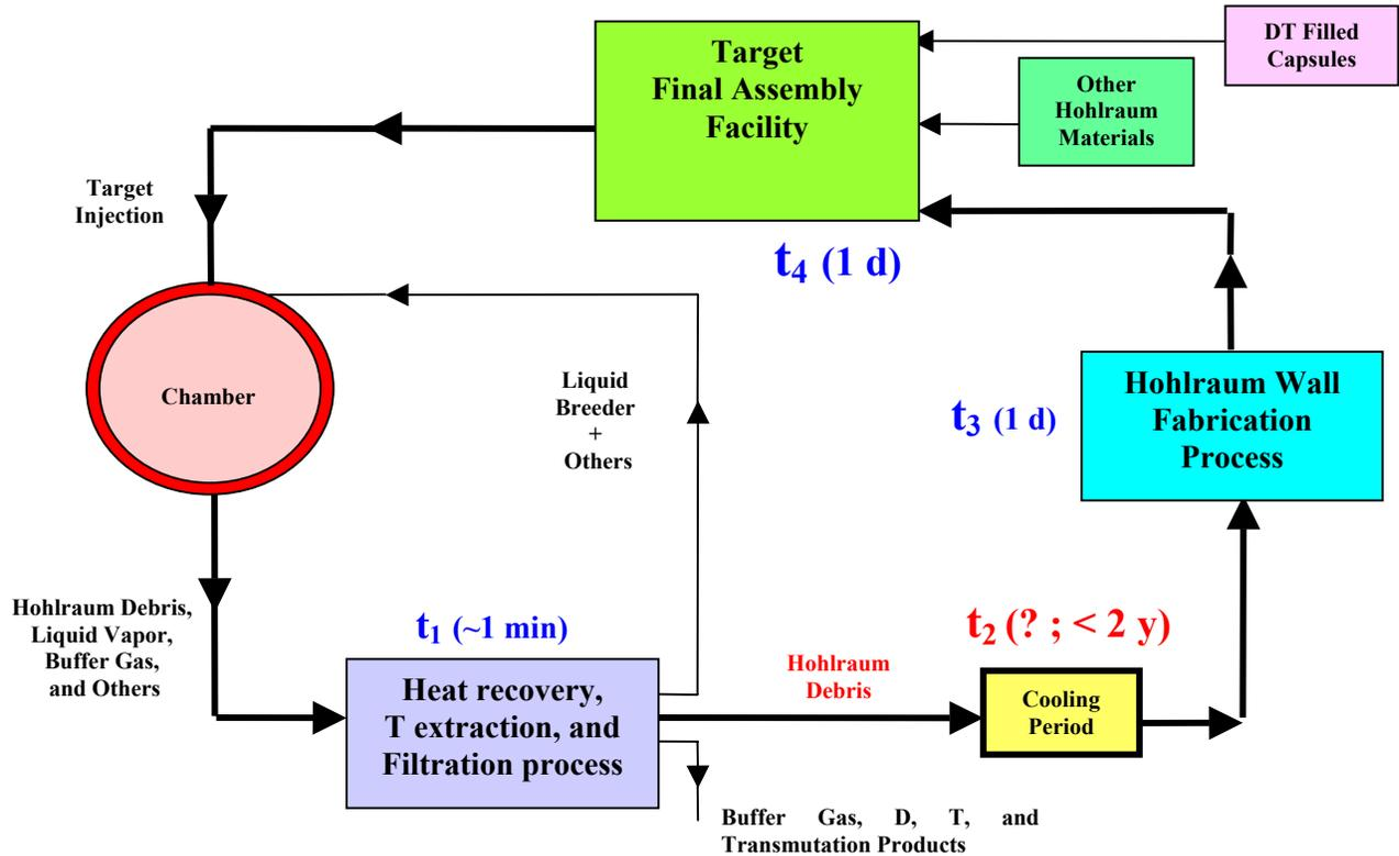
Figure 2. HI target recycling processes and proposed timeline.
