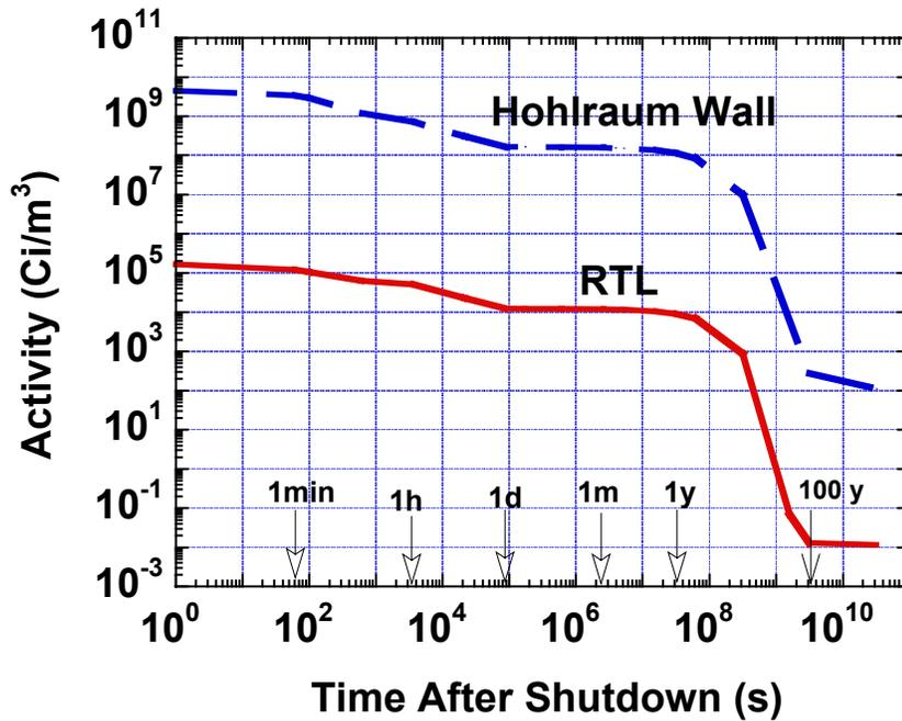
Figure 6. Comparison of activities of hohlraum wall and RTL made out of pure iron.
