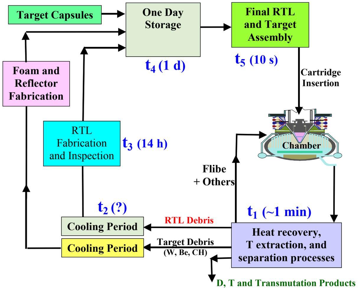
Figure 3. Flow sheet for RTL manufacturing processes and times.
