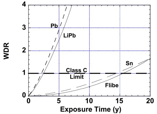
Fig. 3. Increase of liquid film WDR with operation time assuming ~40 min in-chamber residence and no online removal of transmutation products.
