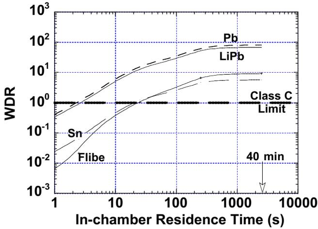
Fig. 2. Variation of liquid film WDR with in-chamber residence time for 47 y of operation without removal of transmutation products.
