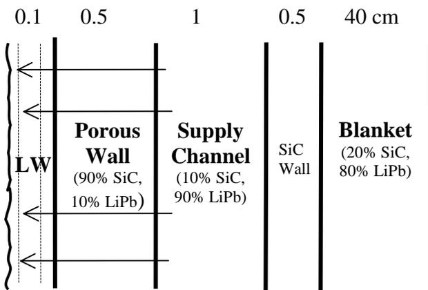
Fig. 1. Representative radial build and typical dimensions of essential components for the porous wall injection scheme (not to scale). A thick LiPb-cooled shield follows the blanket.
