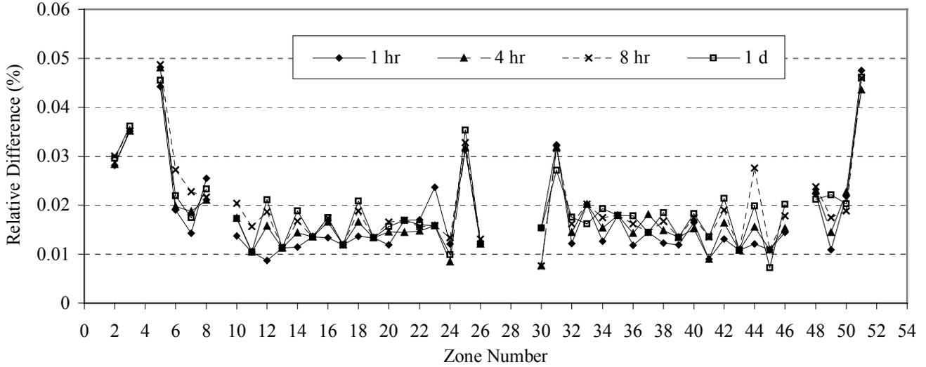
Figure 2. Relative difference (%) between the 100-pulse hybrid approximation and the exact pulsing solution at different cooling times.
