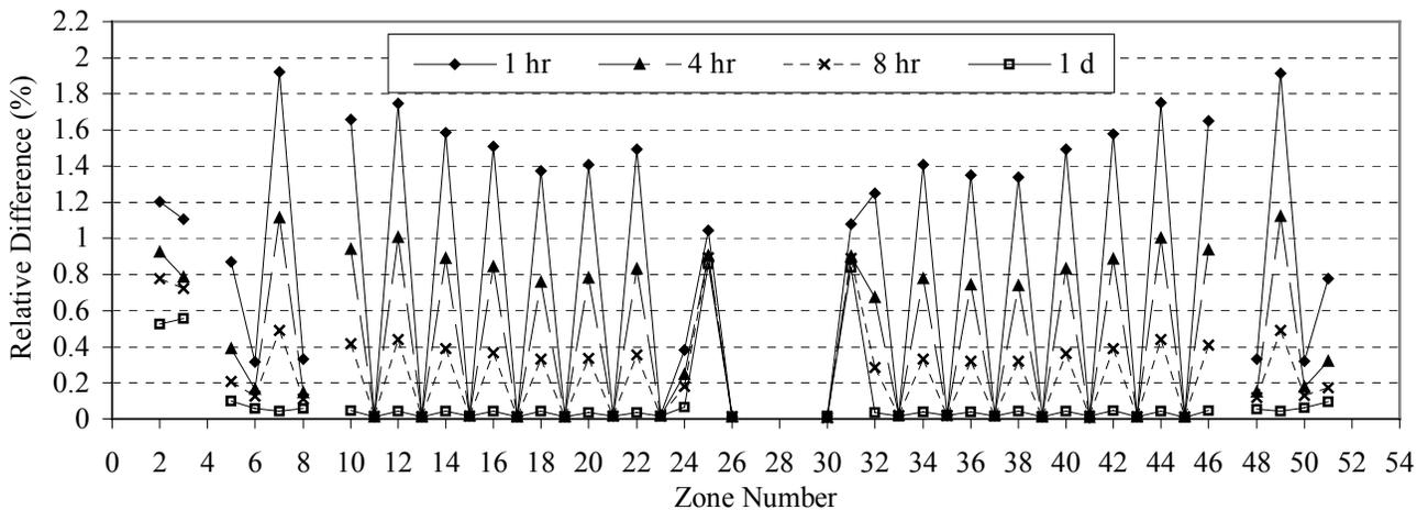
Figure 1. Relative difference (%) between the steady-state approximation and the exact pulse solution at different cooling times.
