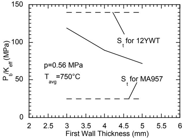
Figure 5. Variation of a Modified Primary Bending Stresses  $P_b/K_{\text{eff}}$  as a Function of FW Thickness.
