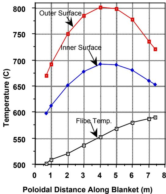
Figure 4. Temperature Profiles as a Function of Poloidal Distance Along the Blanket.
