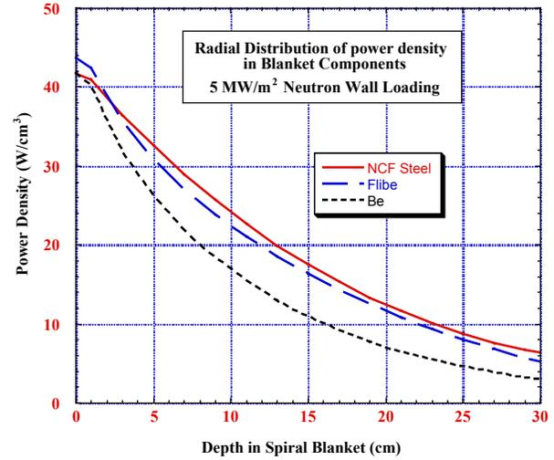
Figure 6. Radial Distribution of Power Density in Blanket Components.
