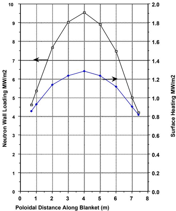
Figure 3. Poloidal Distribution of NWL and Surface Heating.
