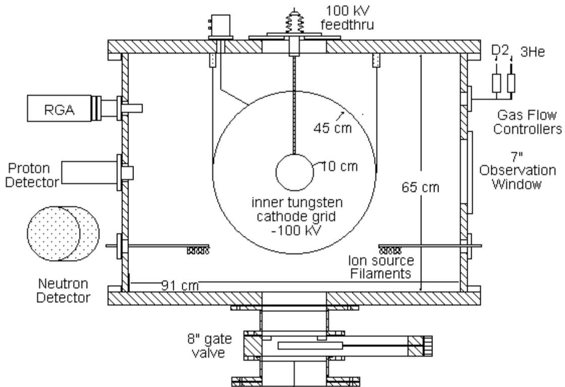
Figure 2. Schematic cross-section through an Inertial Electrostatic Confinement device for laboratory experimentation (courtesy of the Fusion Technology Institute, University of Wisconsin-Madison).
