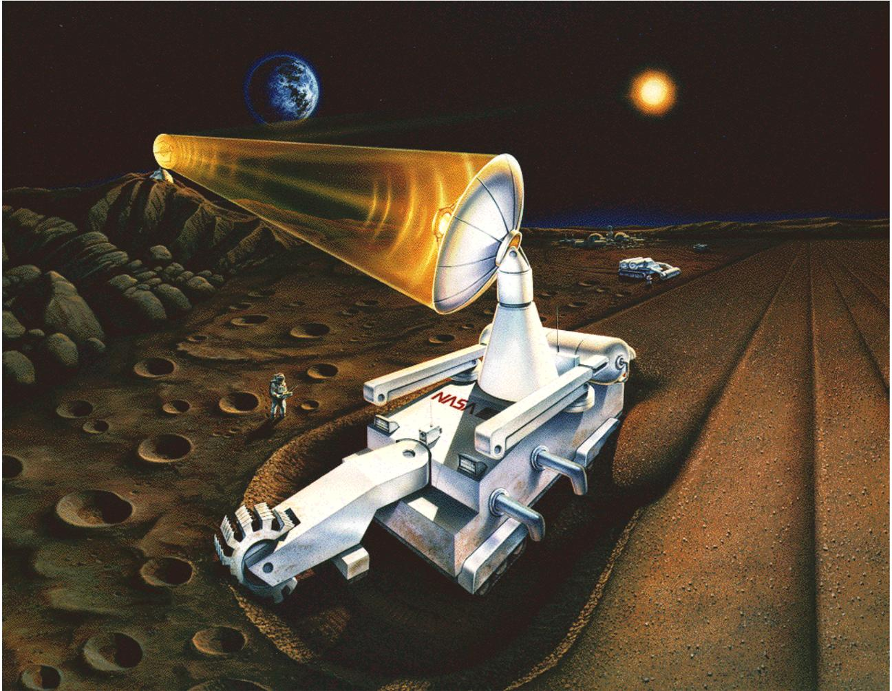
Figure 1. Concept for a mobile mining/processing machine for the extraction of solar wind volatiles, including helium-3, from lunar soils (courtesy of the Fusion Technology Institute, University of Wisconsin-Madison).
