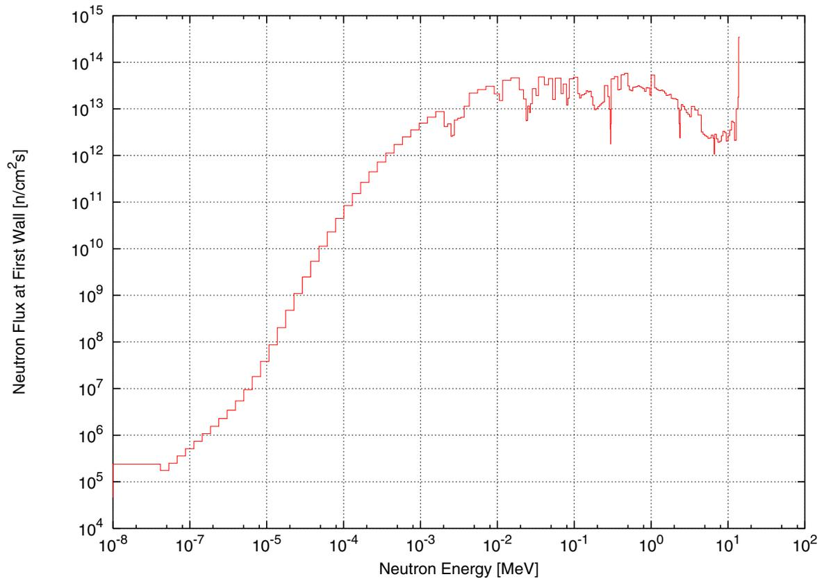
Figure 1. Typical first wall spectrum for advanced tokamak designs with 4 MW/m<sup>2</sup> neutron wall loading (2) [courtesy of P. Wilson (UW)].
