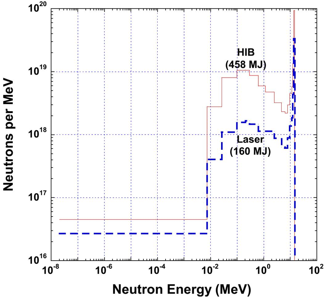
Figure 2. Neutron spectra for ARIES-IFE laser and HIB targets [courtesy of J. Perkins (LLNL)].
