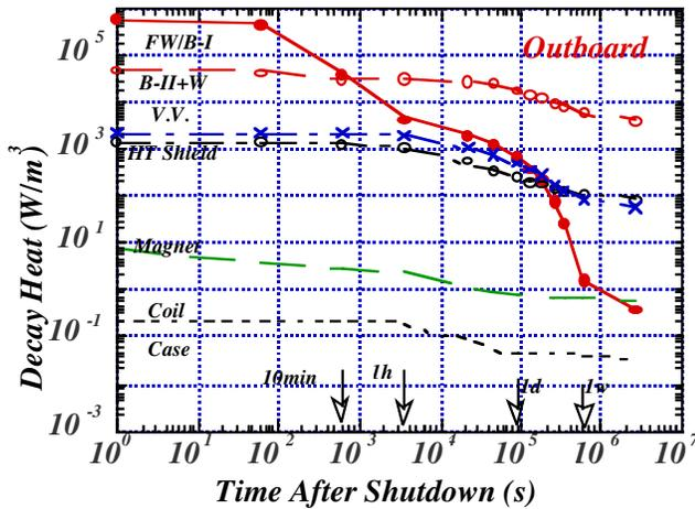
Figure 4. Decay heat of outboard major components.
