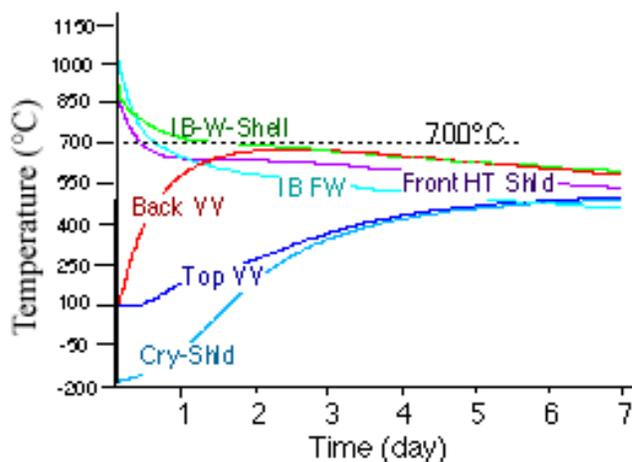
Figure 9. Inboard LOFA temperature history of some key components with cryogenic shield starts at 80 K.
