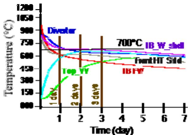
Figure 6. Inboard LOFA temperature history of some key components.
