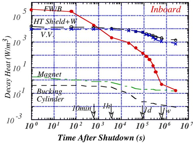
Figure 3. Decay heat of inboard major components.
