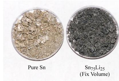
Figure 3: On the left is a photo of the debris that was generated from experiment A-0824 which was pure tin at a volume of 12.25 cc. On the right is a photo of experiment A-0825 Sn<sub>75</sub>Li<sub>25</sub> at a volume of 12.25 cc. Note the the oxidation of the lithium causes a darker dull appearance of the debris.
