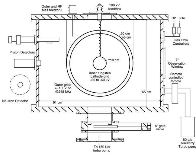
Figure 3. A schematic of the University of Wisconsin IEC device<sup>14</sup> shows the 10 cm diameter inner cathode surrounded by a 50 cm diameter anode. The inner cathode is negatively charged up to 75 kV which attracts the positively charged D<sup>+</sup> and <sup>3</sup>He<sup>+</sup> (and <sup>3</sup>He<sup>++</sup>) formed at the anode by energetic electrons.
