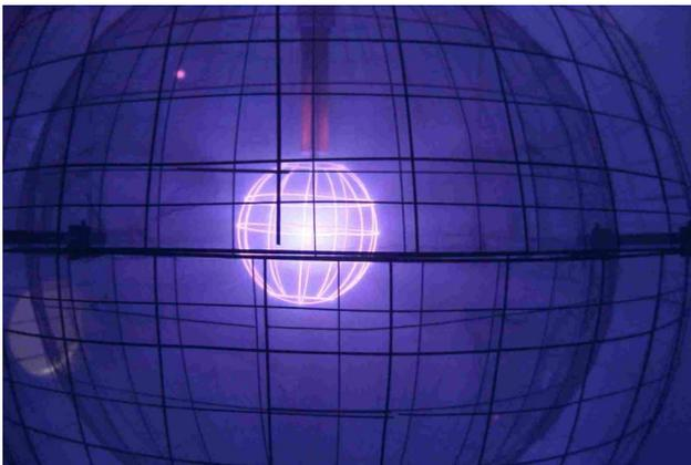
Figure 4. Photograph of a D-<sup>3</sup>He plasma in the center of the Wisconsin IEC device. Currently fusion rates of nearly  $3 \times 10^6$  per second at 55 kV and a current of 60 mA have been achieved.
