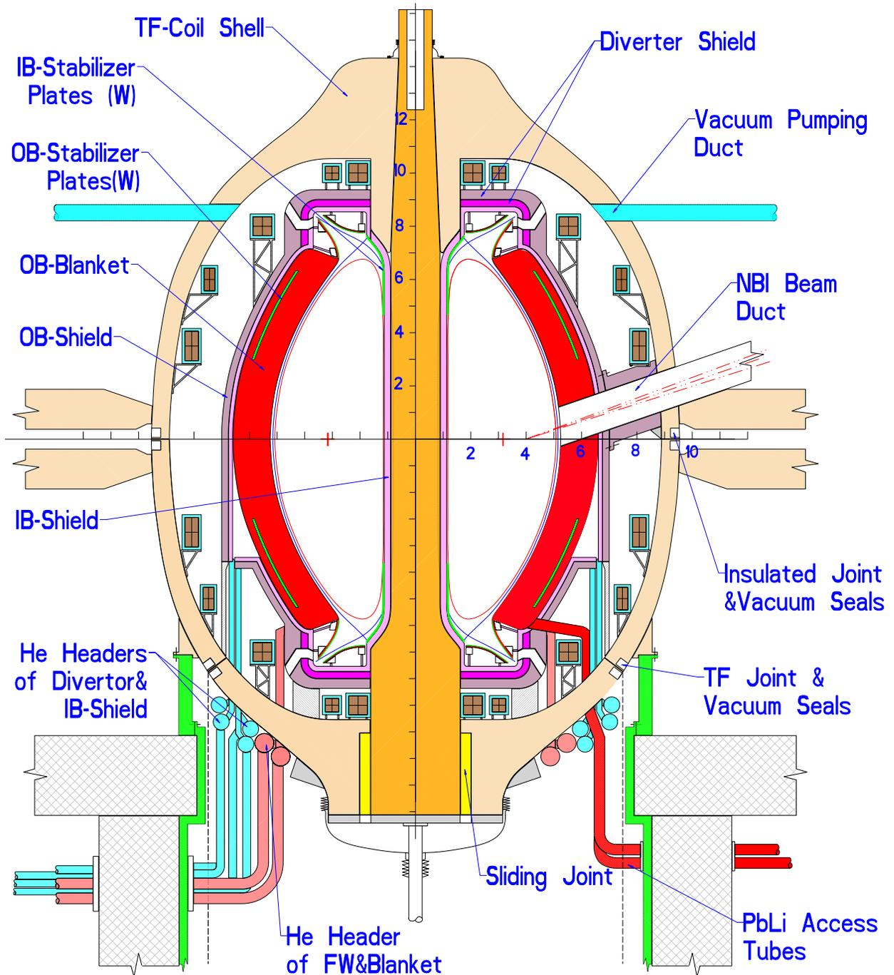
Figure 1. Vertical cross-section of ARIES-ST.
