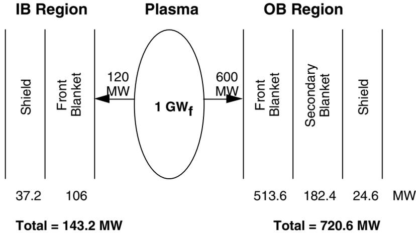
Fig. 6. Nuclear heating partitioning in the reference EVOLVE design.
