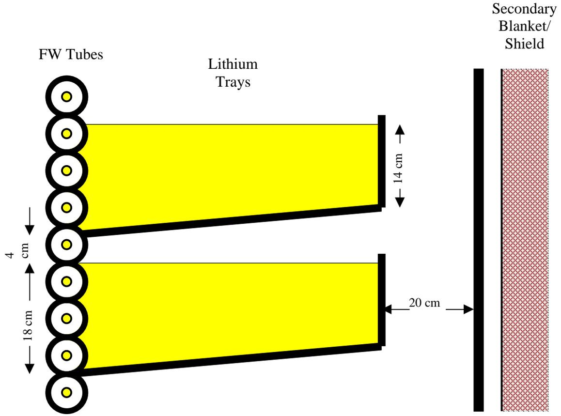
Fig. 1. Configuration of the EVOLVE FW/blanket concept.
