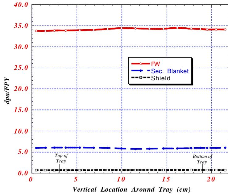
Fig. 8. Poloidal variation of damage rate around an OB tray.
