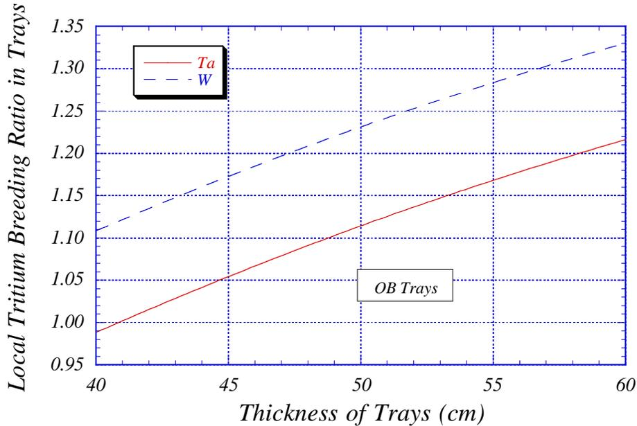
Fig. 2. Impact of structural material on local TBR.
