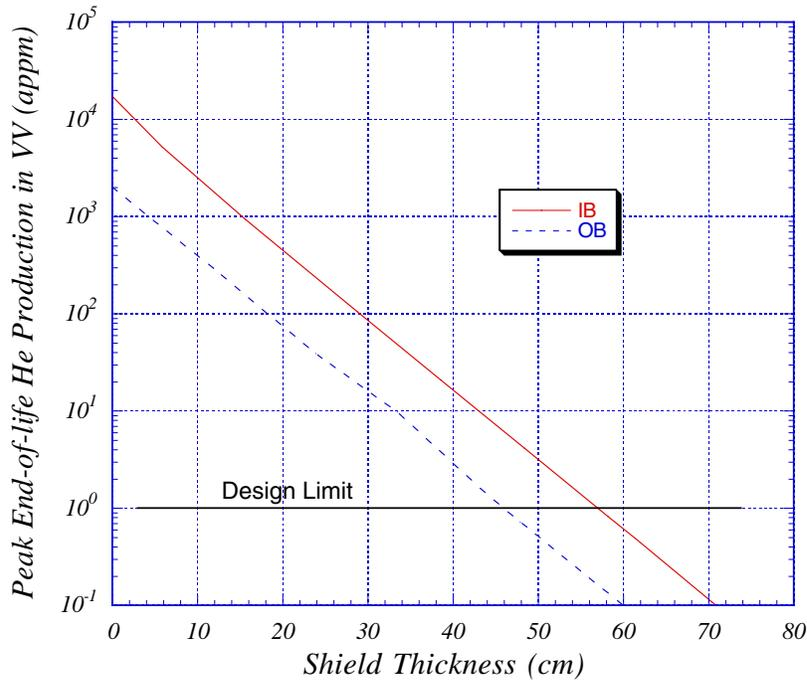
Fig. 4. Effect of shield thickness on peak end-of-life helium production in the VV.
