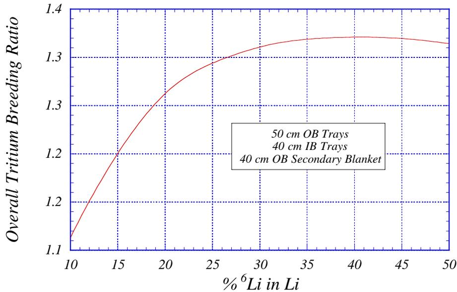
Fig. 3. Effect of Li enrichment on overall TBR.
