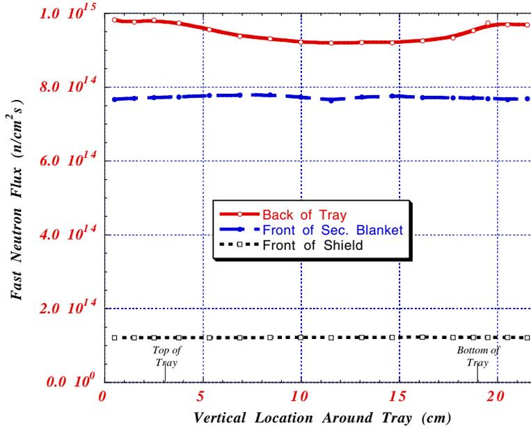
Fig. 7. Poloidal variation of fast neutron flux.
