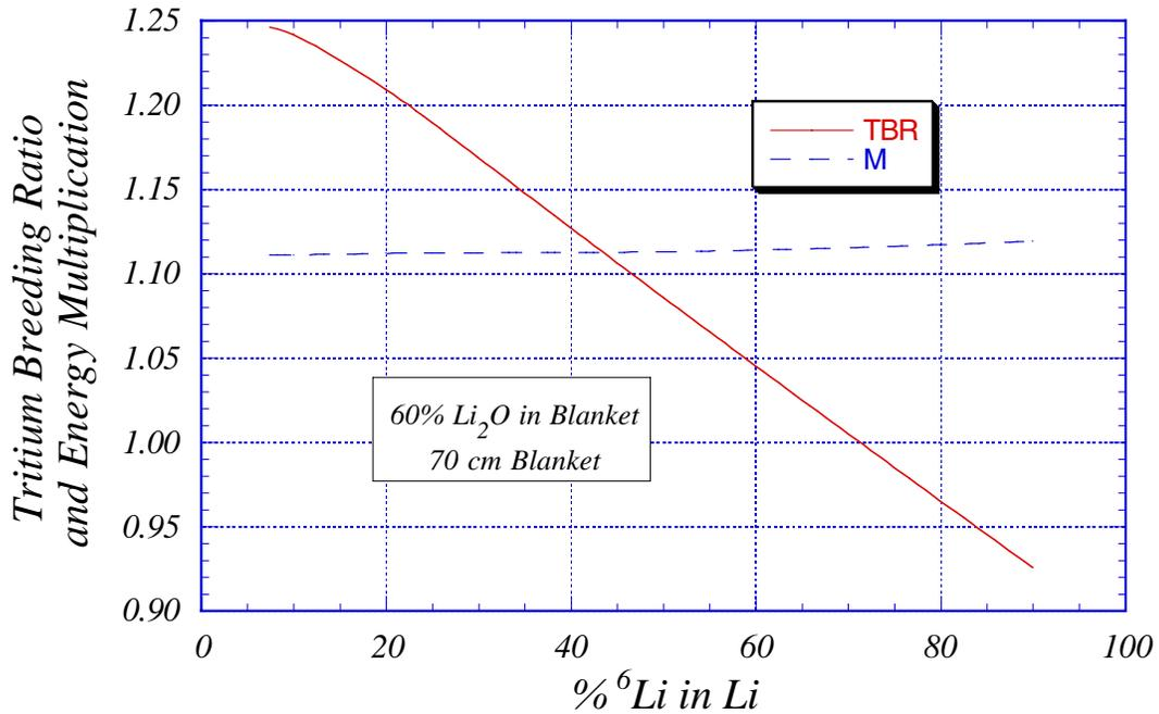
Fig. 3. Effect of lithium enrichment on local TBR and energy multiplication.
