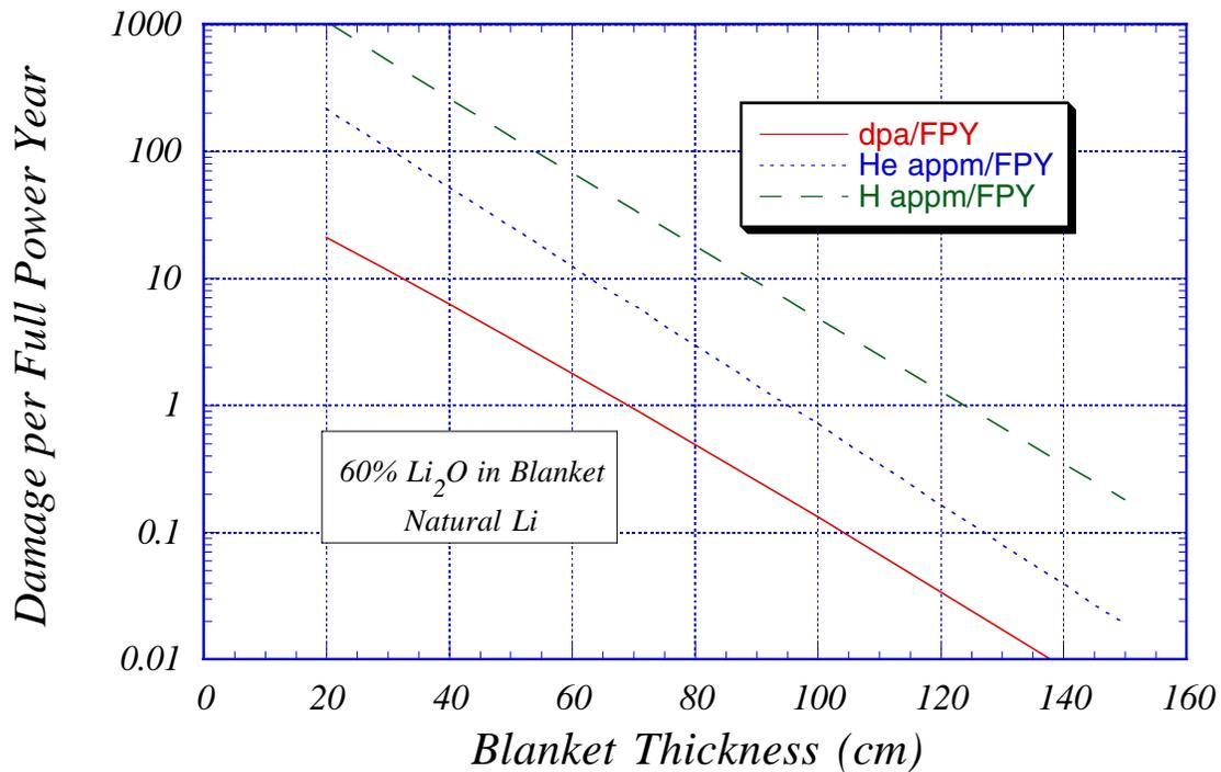
Fig. 4. Impact of blanket thickness on peak damage and gas production rates in the steel structure of the shield.
