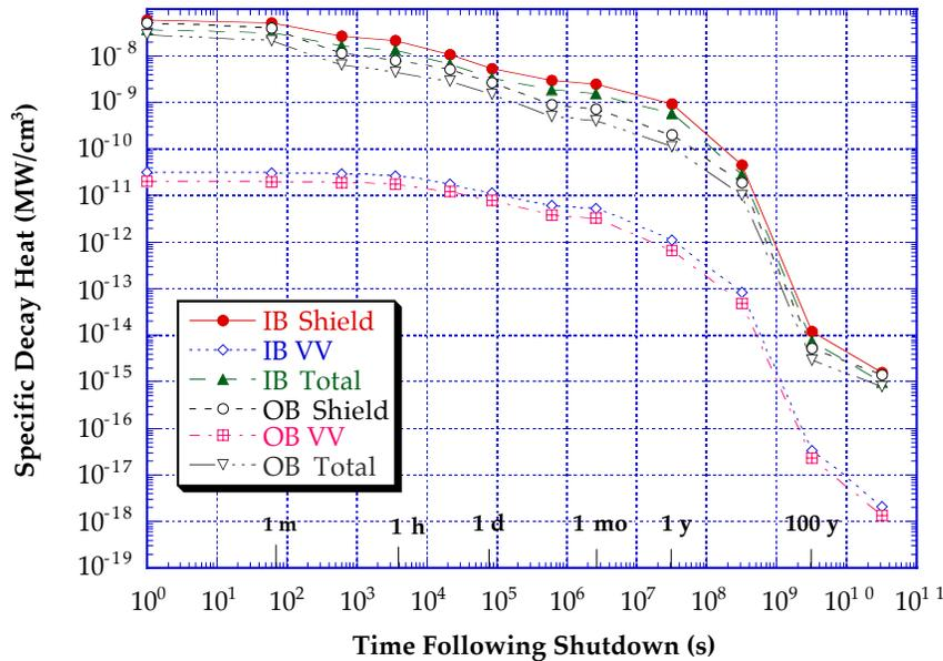
Fig. 7. Decay heat induced in the different components as a function of time following shutdown.
