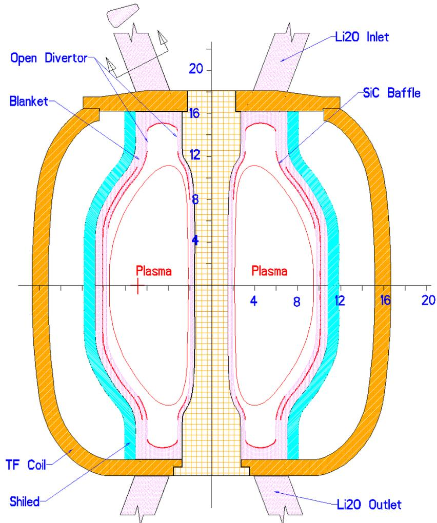
Fig. 1. Schematic of the APPLE concept.
