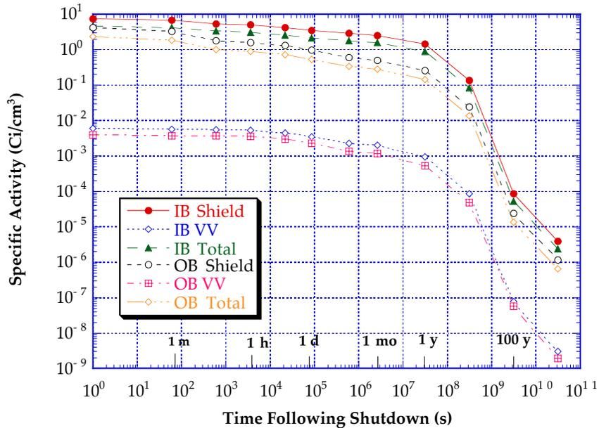
Fig. 6. Activity induced in the different components as a function of time following shutdown.
