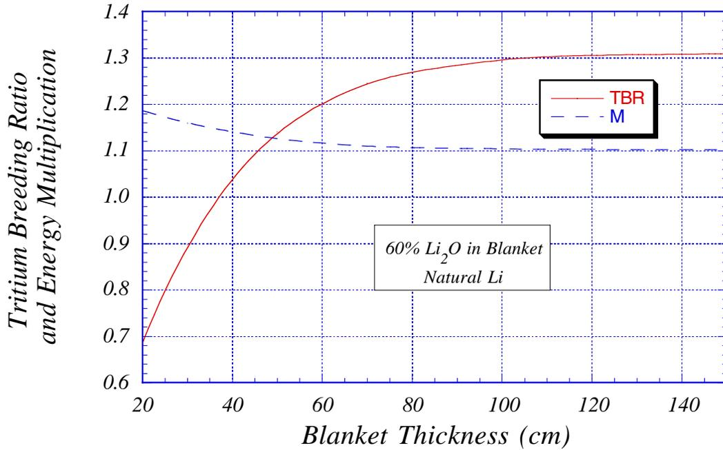
Fig. 2. Impact of blanket thickness on local TBR and energy multiplication.
