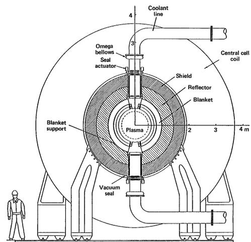
Figure 2: *Cross section of the MARS tritium-breeding blanket.*
