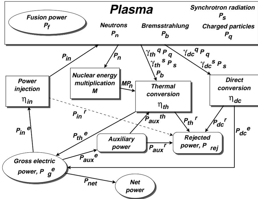
Figure 3: FRC plasma and plant power flow.
