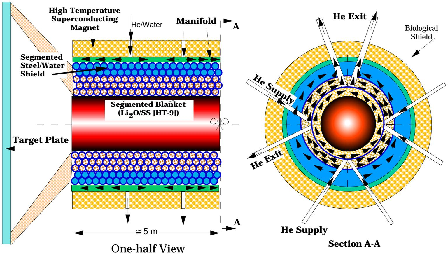
Figure 2: One-half view and cross section of a preliminary concept for the tritium-breeding blanket.
