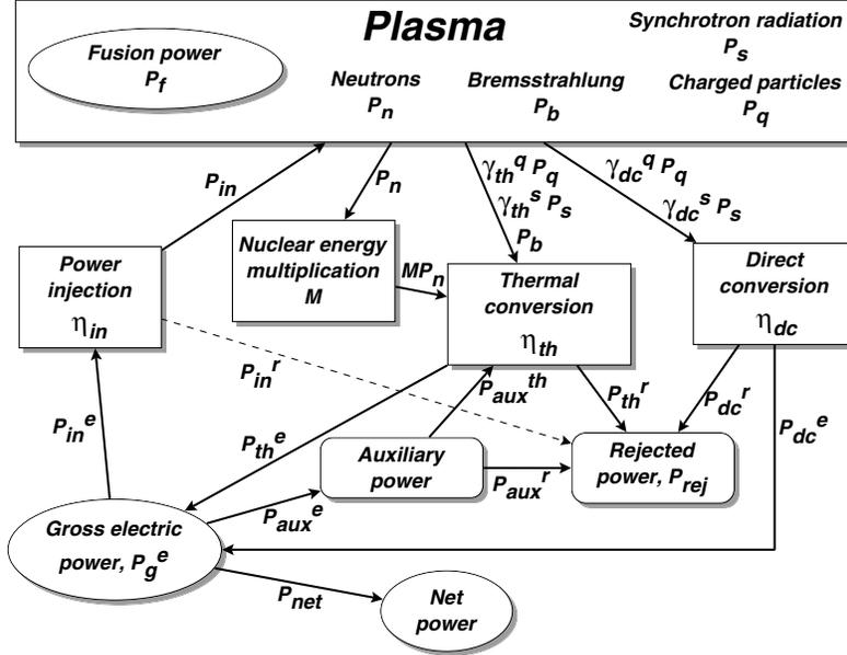
Figure 1: *FRC plasma and plant power flow.*
