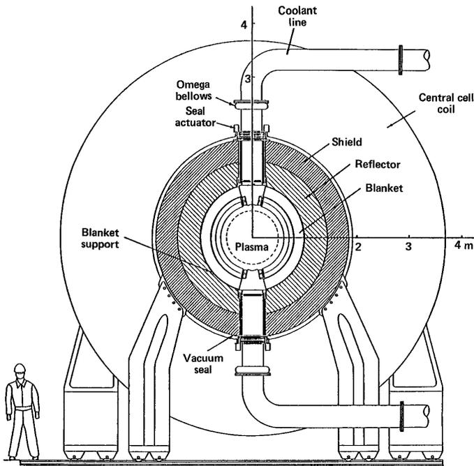
Figure 3: Cross section of the MARS tritium-breeding blanket.
