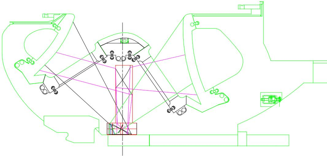
Fig. 2. The central diagnostic cassette showing the viewing slots and mirrors.
