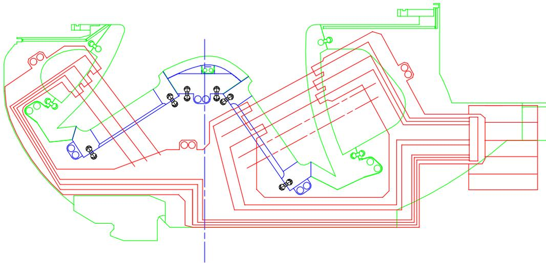
Fig. 3. The central diagnostic cassette showing the waveguide panel.
