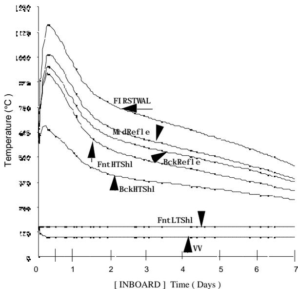
Figure 5. A general temperature variation history during the first week after shutdown of the inboard.
