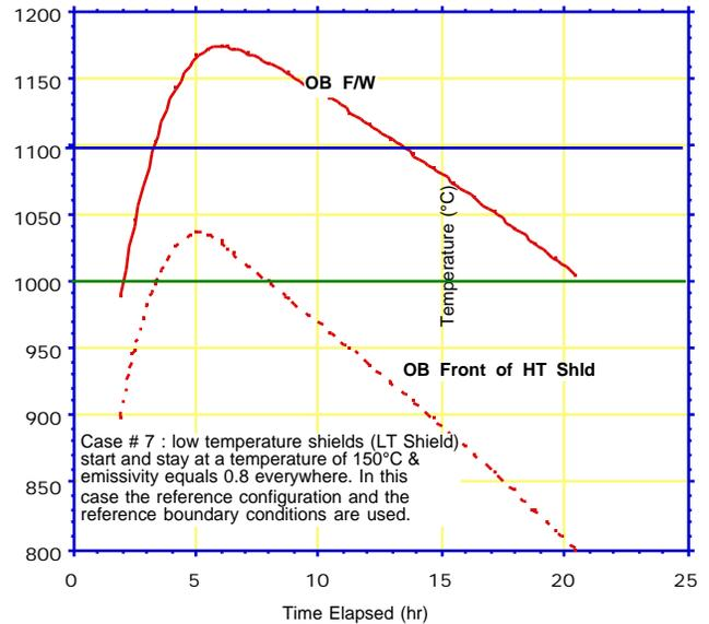
Figure 4. Temperature variation of the first wall and the front of the hot temperature shield for the final case (Case #7).
