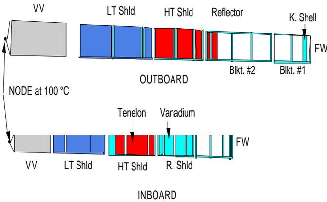
Figure 1. Finite element model for the inboard and the outboard of ARIES-RS.
