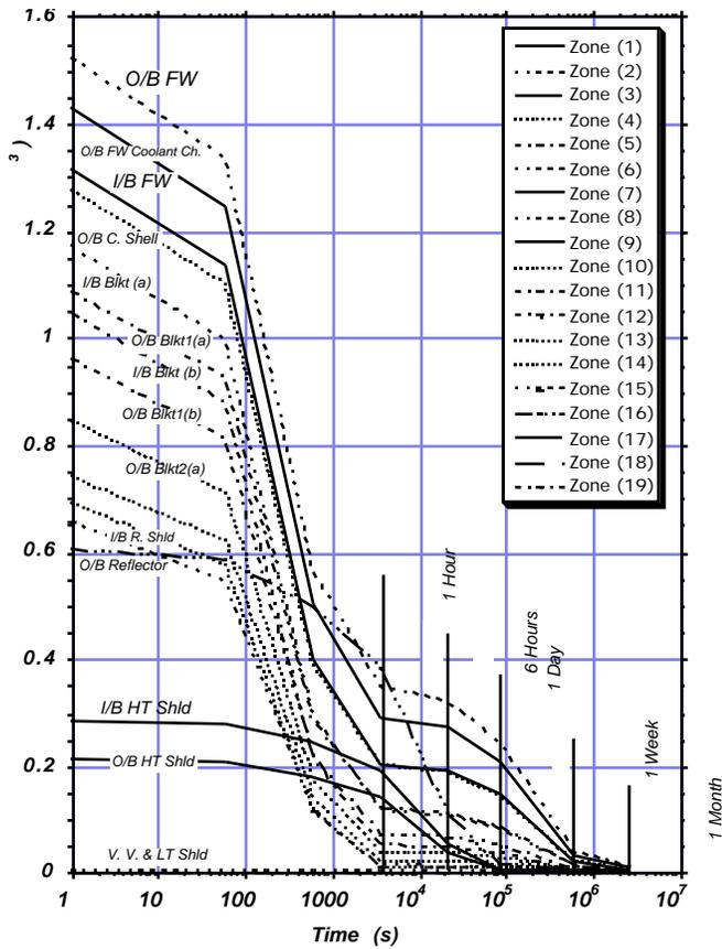
Figure 2. Specific afterheat in a 100% dense material (Tenelon in O/B reflector) (reference case).
