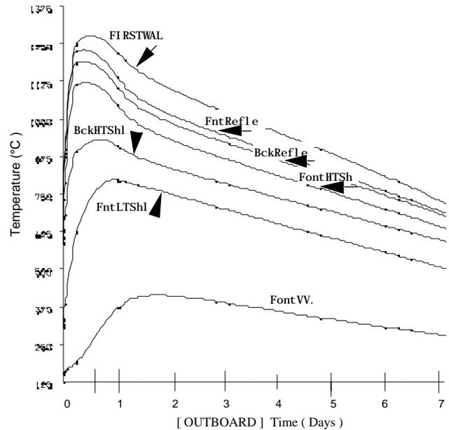
Figure 6. A general temperature variation history during the first week after shutdown of the outboard.
