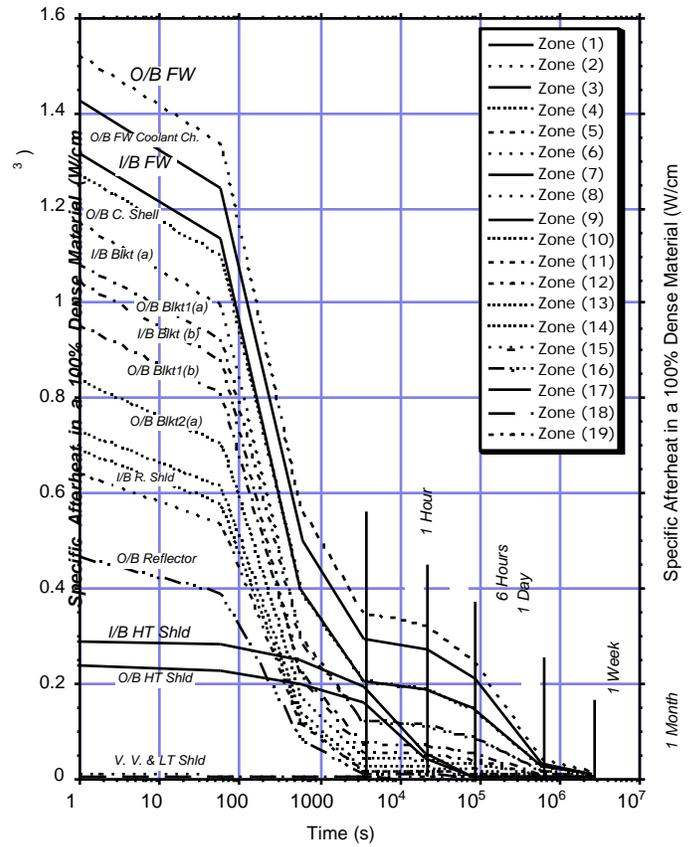
Figure 3. Specific afterheat in a 100% dense material (vanadium in O/B reflector).
