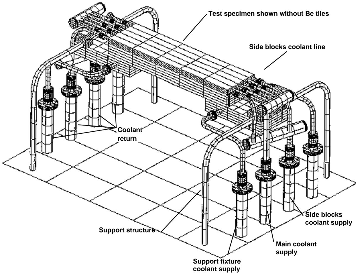
Figure 2. Test bed for the ITER small scale limiter specimen.
