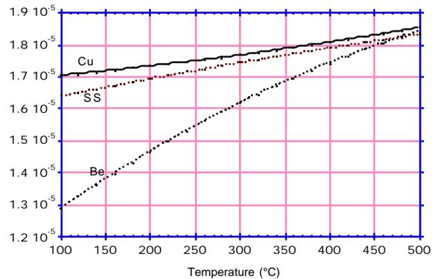
Figure 3. Comparison of the coefficient of thermal expansion for Cu, SS, and Be.
