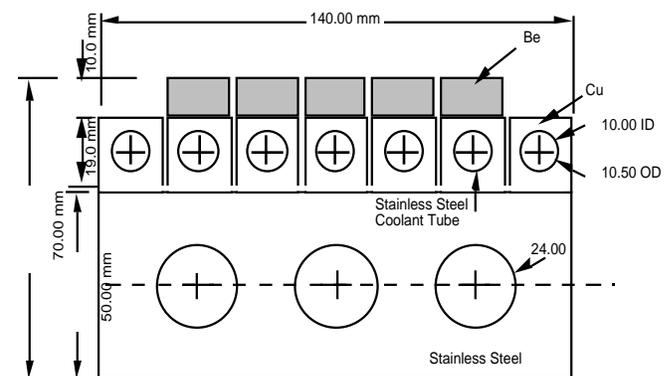
Figure 1. The small scale specimen for the ITER limiter.
