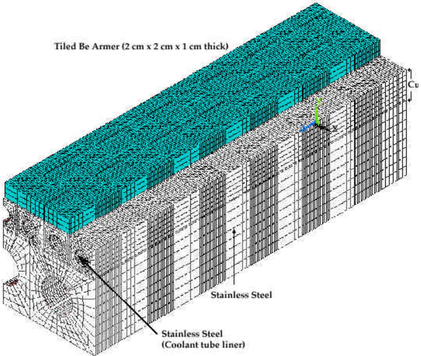
Figure 4. The 3-D finite element model.
