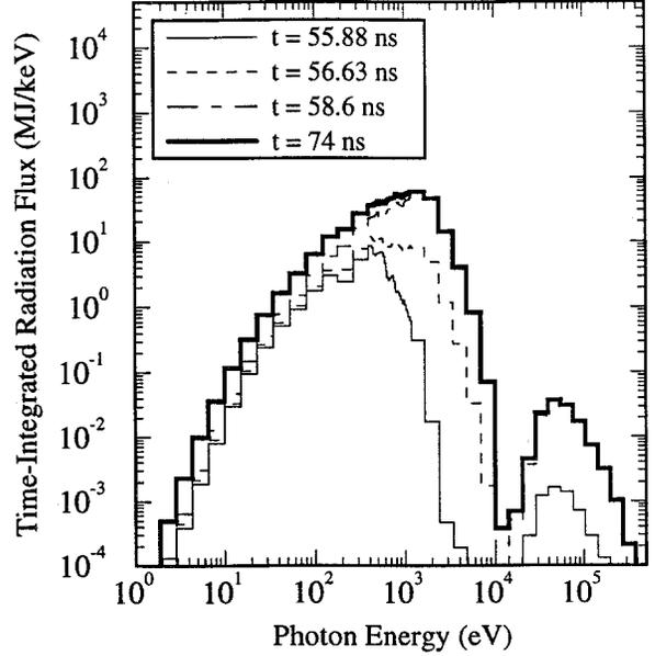
Fig. 4. Frequency dependence of radiation energy emitted from the target. Results are time-integrated up to simulation times shown.
