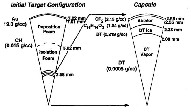
Fig. 1. Schematic illustration of initial target configuration for LIBRA-SP.
