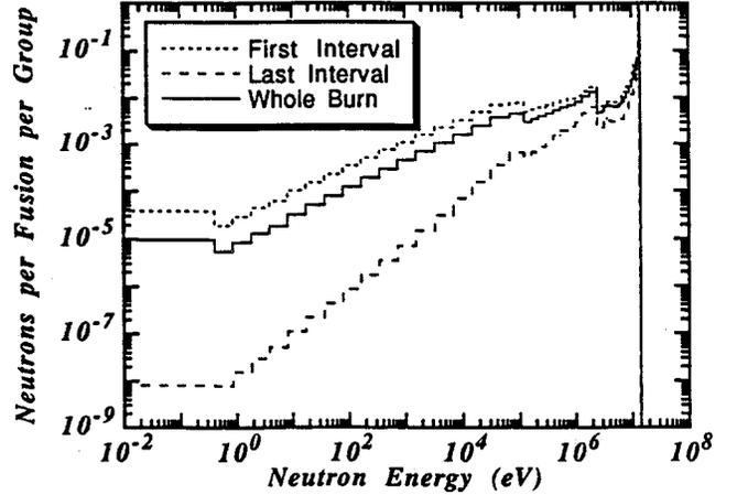
Fig. 5. Energy spectrum of neutrons emitted from the LIBRA-SP target.
