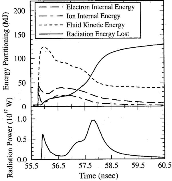
Fig. 2. (Top) Energy partitioning vs. simulation time. The fusion burn phase occurs between  $t = 55.7$  and  $55.9$  ns. (Bottom) Time dependence of x-ray radiation power escaping the target.
