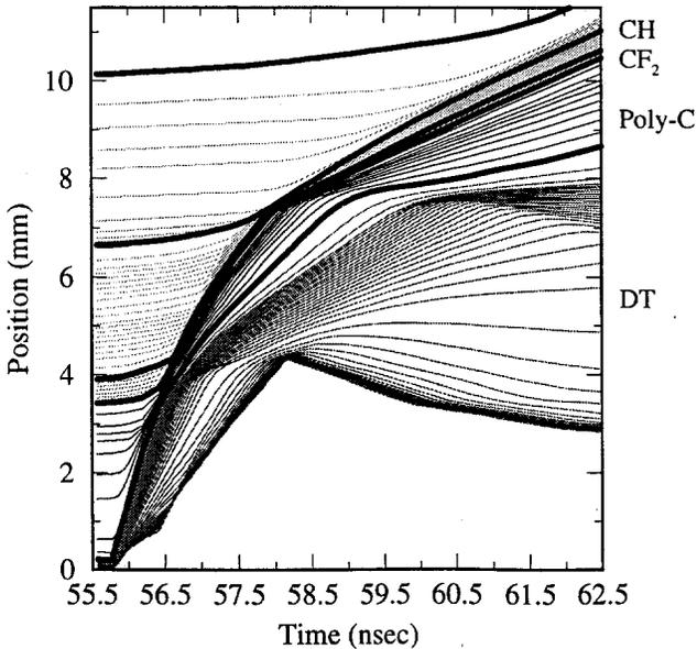
Fig. 3. Lagrangian zone boundary conditions vs. time. The thick solid curves indicate the interfaces between different materials.
