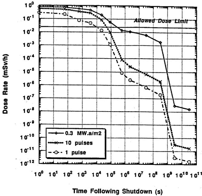
Fig. 3. Biological dose rates behind the cryostat.
