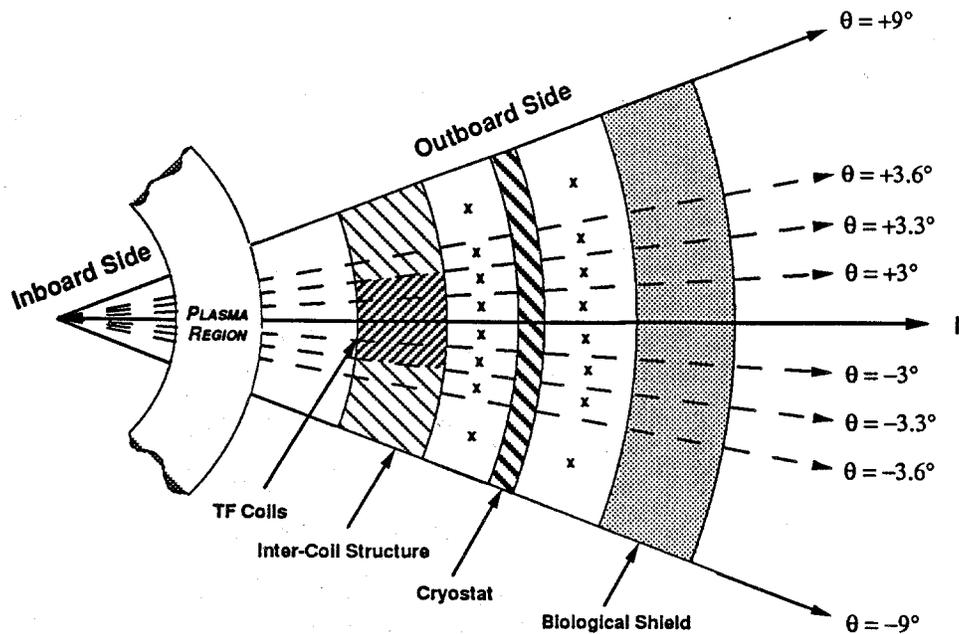
Fig. 1. Schematic of the two-dimensional  $r$ - $\theta$  model.
