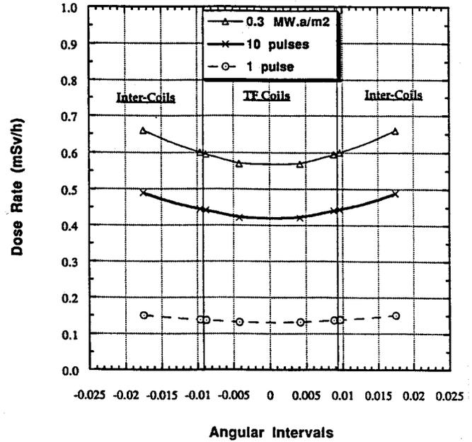
Fig. 4. Biological dose rates at shutdown behind TF coils as a function of angular intervals.
