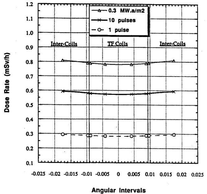
Fig. 5. Biological dose rates at shutdown behind cryostat as a function of angular intervals.
