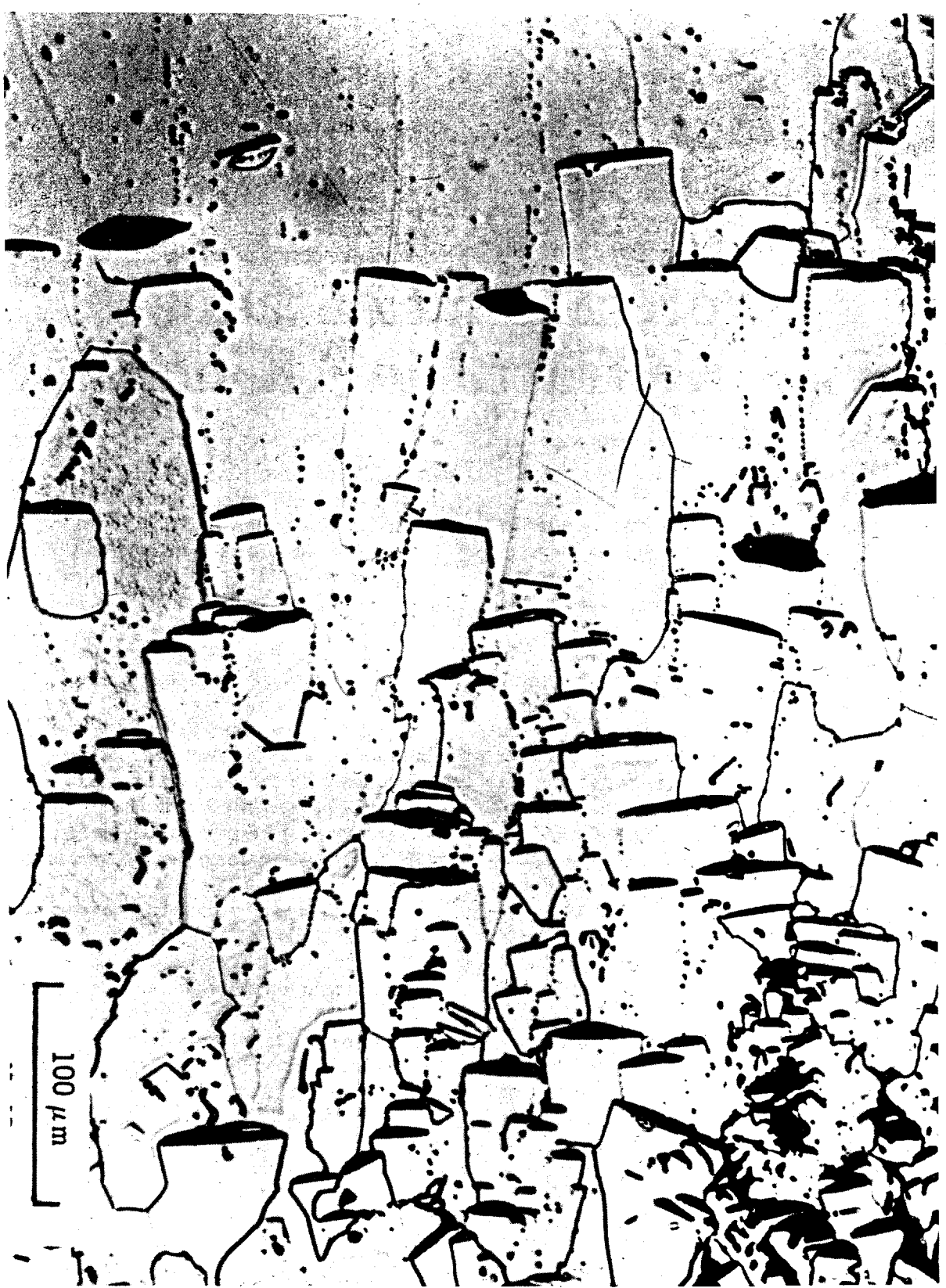
Fig. 14.1 Lenticular pores migrating up the temperature gradient in \text{UO}_2 . The temperature increases from bottom to top. (Courtesy of J. R. MacEwan and V. B. Lawson, Atomic Energy of Canada, Ltd.)
