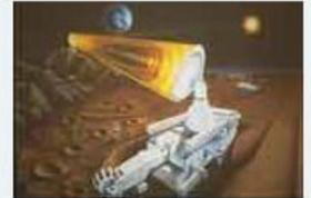
A possible design for a rover to extract helium-3 from the lunar soil. The robot would capture sunlight, reflected from a gathering dish, to bake the soil. Credit: University of Wisconsin
